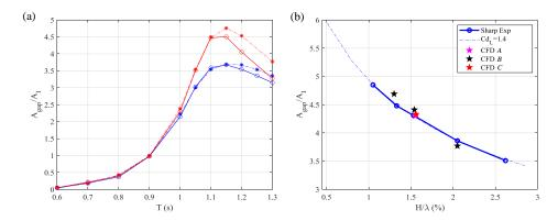
FIGURE 3. Free surface RAOs; (a) as function of wave period for constant wave steepness of  $H/\lambda = 1.3\%$  (blue) and 2.6% (red), with the dashed-line corresponding to the damping-lid model prediction; (b) as a function of wave steepness for  $T=1.1\mathrm{s}$  with results for both the lid damping model and CFD shown.
