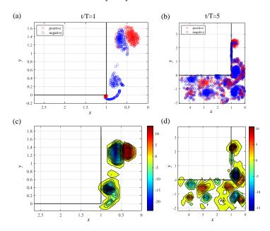
FIGURE 16. Discrete vortex distributions (a, b) and corresponding vorticity contours (c, d) for t/T = 1 and t/T = 5.
