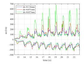
FIGURE 10. Comparison of the measured vorticity maxima using different field of views and pixel sizes for  $T = 1.1 \,\mathrm{s}$  and  $H/\lambda = 1.6 \,\%$ .
