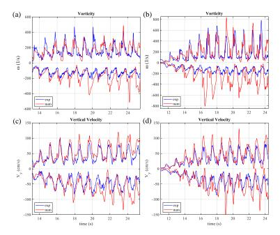
FIGURE 12. Comparison of the computed and measured vorticity and vertical velocity maxima for  $T = 1.1 \,\mathrm{s}$  and  $H/\lambda = 1.6 \,\%$ . (a,c) PIV with pixels of  $0.071 \,\mathrm{mm}$  (case III) and CFD with a mesh size of  $dx = 0.50 \,\mathrm{mm}$  (case B); (b,d) PIV with pixels of  $0.037 \,\mathrm{mm}$  (case IV) and CFD with a mesh size of  $dx = 0.25 \,\mathrm{mm}$  (case C).
