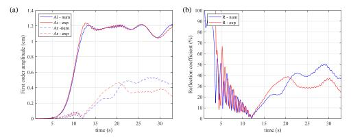
FIGURE 5. (a) Time evolution of the incident and reflected waves amplitudes and (b) reflection coefficients, obtained using the separation method for T = 1.1s and  $H/\lambda = 1.3\%$ .
