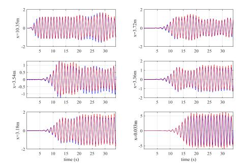
FIGURE 4. Time histories of the measured (blue) and CFD prediction (red) of the free surface elevation (in cm) at various distances upstream from the vertical wall, for  $T=1.1\,\mathrm{s}$  and  $H/\lambda=1.3\,\%$ .
