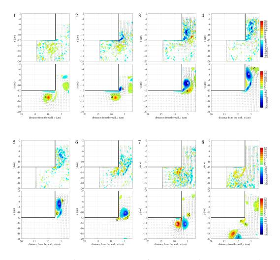
FIGURE 6. Measured (upper panels, for case II) and computed (lower panels, case A) instantaneous vorticity contours at equivalent intervals of T/8 (numbered consecutively) during resonance for  $H/\lambda = 1.6\,\%$ ,  $T = 1.1\,\mathrm{s}$ . The vortex cores are labelled A to E. The extent of the PIV field of view is shown by the dashed lines.
