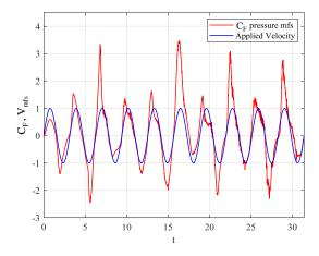
Figure 17. Force coefficient time history computed using DVM.
