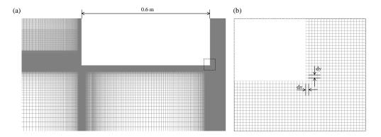
FIGURE 2. CFD mesh; (a) in the region of the hull and wall and (b) in the region of the bilge edge in the gap (bounded by dashed-lines in (a)).
