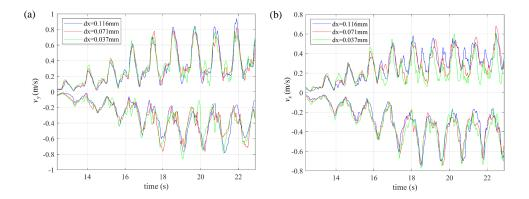
FIGURE 11. Comparison of the measured (a) vertical (b) horizontal velocity maxima using different field of views and pixel sizes for  $T = 1.1 \,\mathrm{s}$  and  $H/\lambda = 1.6 \,\%$ .
