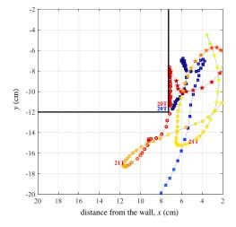
FIGURE 14. Trajectories from formation of the vortices 'A' ( $\circ$ ), 'B' ( $\square$ ), 'C' ( $\star$ ), as identified in figure 13. The vorticity colour range is consistent with figure 6 and the positions of the vortices at time t = 20T and 21T are labelled for reference.
