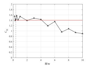
FIGURE 18. Vortex drag coefficient dependency computed using DVM. The continuous red line indicates the empirical value of  $C_D$  used for the damping lid model computations. The dashed line corresponds to the value of H/w for the experiment, damping lid model and CFD results.
