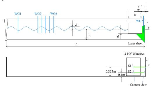
FIGURE 1. Experimental arrangement in the wave tank.
