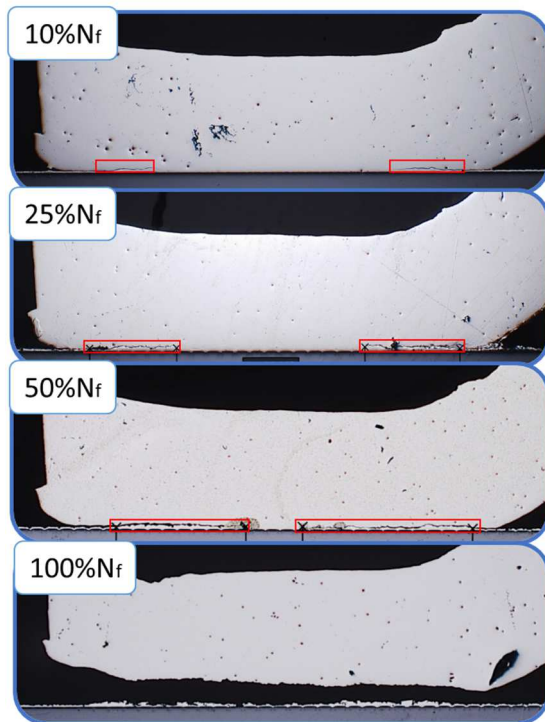
Fig.19 : The crack propagation for samples degraded at 10% N_f , 25% N_f , 50% N_f and 100% N_f .
