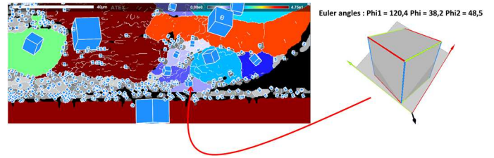
Fig.4 : Grains orientations and Euler indices representing their orientation angles at the heel position.
