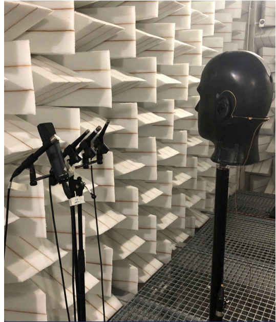
TESTING MICROPHONES FOR CROSS-TALK REJECTION IN THE ANECHOIC CHAMBER
