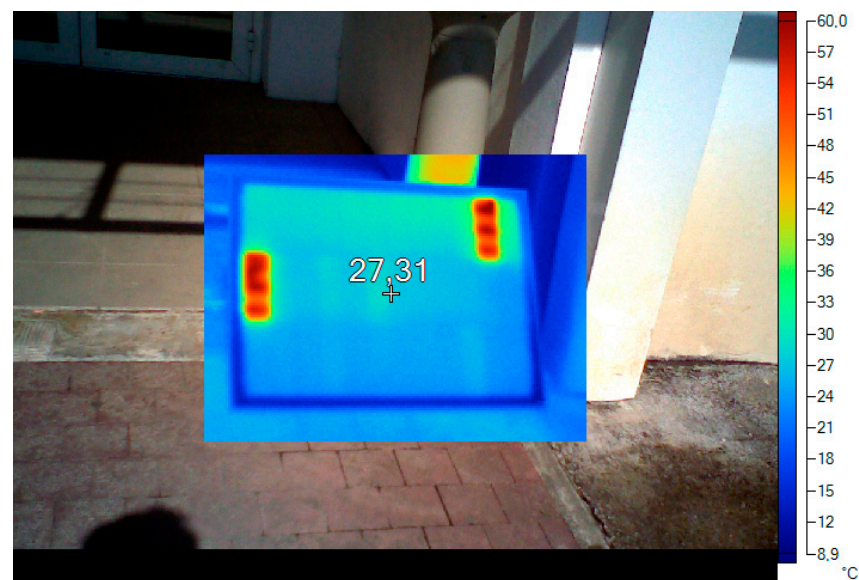
Figure 13. Thermal images of the panel exposed to sunlight. Cell 12 and Cell 212 are significantly hotter than the rest.
