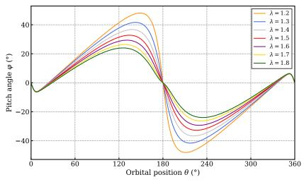
Figure 5 – Optimized pitch laws for different  $\lambda$  values in case of thrust maximization
