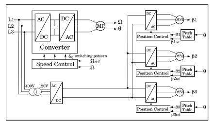
Figure 9 – Electrical diagram of the experimental thruster
