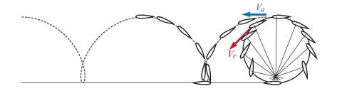
**Figure 1** – 2D blade path for the epicycloid mode ( $\lambda < 1$ )
