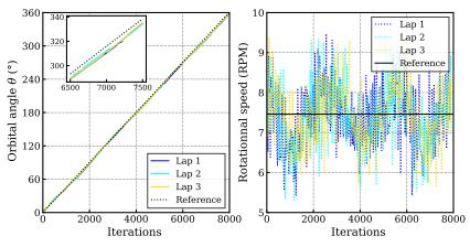
**Figure 10** – Measured orbital position  $\theta$  and rotational speed during three laps
