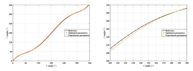
**Figure 12** – Blade-control comparison on  $\beta$  between experiments controller parameters and Matlab Simulink parameters. At the right, zoom on the x-axis.
