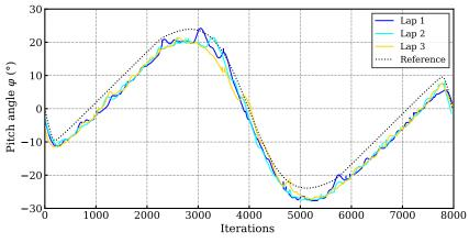
**Figure 11** – Pitch law  $\varphi$  measured during three laps
