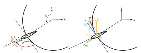
Figure 4 – Angle definitions (left) and hydrodynamic force decomposition (right) for an arbitrary position  $\theta$
