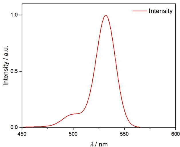
Figure 6. Simulated vibrationally resolved absorption spectrum for tautomer **B**, calculated at TI VG|FC level and using B3LYP-D3 as density functional and 6-31+G(d,p) as basis set. The acetonitrile solvent effects have been taken into account by using PCM implicit solvation method. A Gaussian distribution of  $350\text{ cm}^{-1}$  has been used to simulate the broadening.
