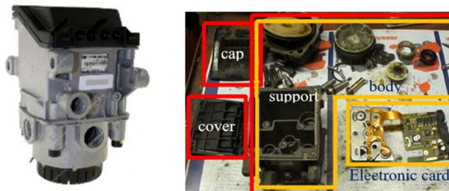
Figure 11 EBS module and components of the returned module [12]
