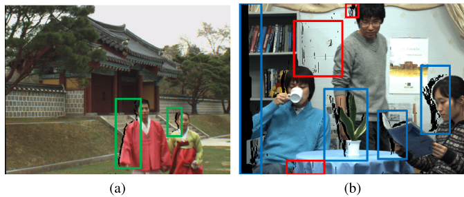
Fig. 4. Examples of typical dis-occluded/missing regions introduced during the process of DIBR based views synthesis. (a) Examples of dis-occluded regions that are around foreground objects' boundaries (bounded by green boxes); (b) Examples of small and medium size of textureless regions (bounded by red and blue bounding boxes correspondingly) that distributed throughout the image.
