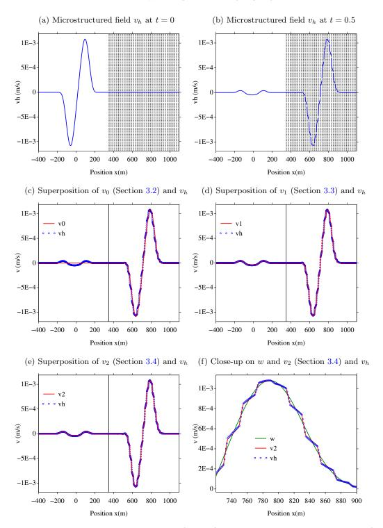
Figure 3. Wave in a homogeneous half-space (a-b, left) impacting a microstructured half-space (a-b, right) with impedance matching  $(E_{-}\rho_{-}=E_{0}\rho_{0})$ . The central frequency is  $f_{c}=3$  Hz ( $\varepsilon_{c}=0.043$ ).
