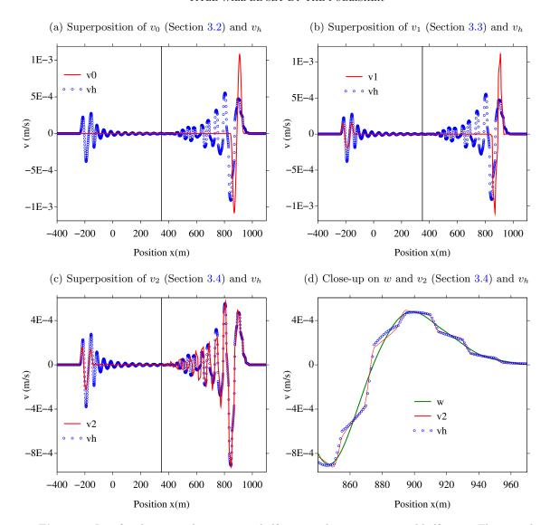
Figure 5. Interface between a homogeneous half-space and a microstructured half-space. The central frequency is  $f_c = 12$  Hz ( $\varepsilon_c = 0.172$ ), and time is t = 0.5.
