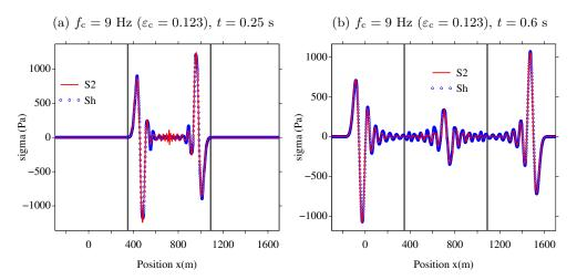
Figure 10. Wave emitted by a source point in a heterogeneous slab: comparisons between "total" stress  $\sigma_2$  (Section 3.4) and the microstructured field  $\sigma_h$  at central frequency  $f_c = 9$  Hz (central row of Figure 9), represented at t = 0.25 (a) and t = 0.6 (b).
