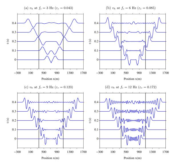
Figure 8. Waves emitted in a microstructured slab surrounded by two homogeneous half-spaces: microtructured velocity  $v_h$  for several source frequency and times. For the clarity of the figure, the internal interfaces are not shown.
