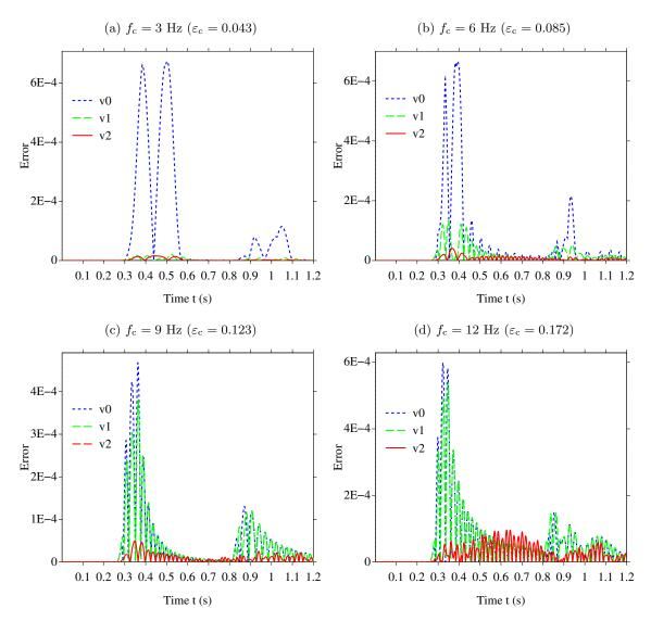
**Figure 11.** Waves emitted in a microstructured slab sourrounded by two homogeneous half-spaces. Time evolution of the errors  $|v_h(x_r,t)-v_n(x_r,t)|$  at receiver  $x_r$ , with the orders n=0,1,2.
