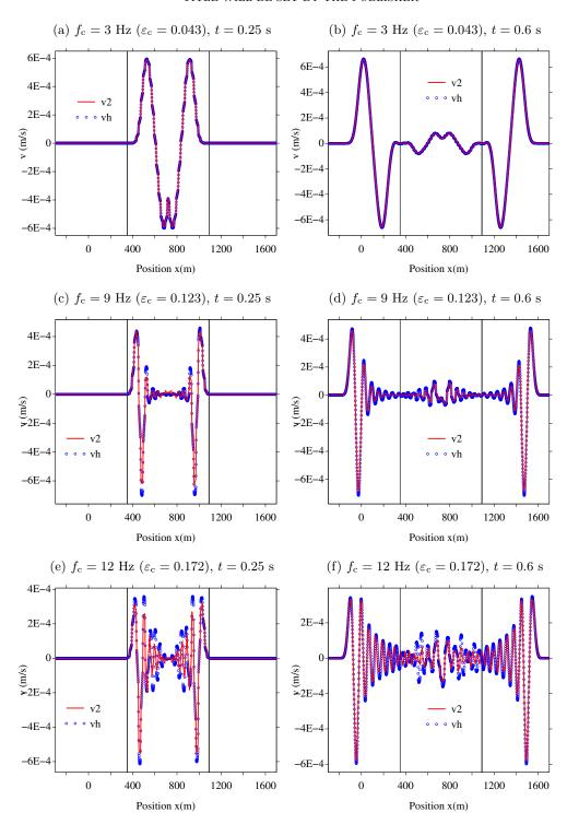
Figure 9. Wave emitted by a source point in a heterogeneous slab: comparisons between "total" velocity  $v_2$  (Section 3.4) and the microstructured field  $v_h$  at three central frequencies (rows), represented at t = 0.25 (left column) and t = 0.6 (right column).
