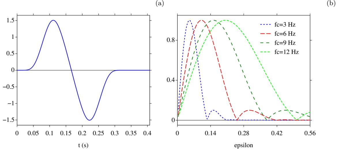
**Figure 2.** Time evolution of the source (58) at  $f_c = 3$  Hz (a). Spectrum of the source for various central frequencies  $f_c$ , as a function of the asymptotic parameter  $\varepsilon_c$  (b).
