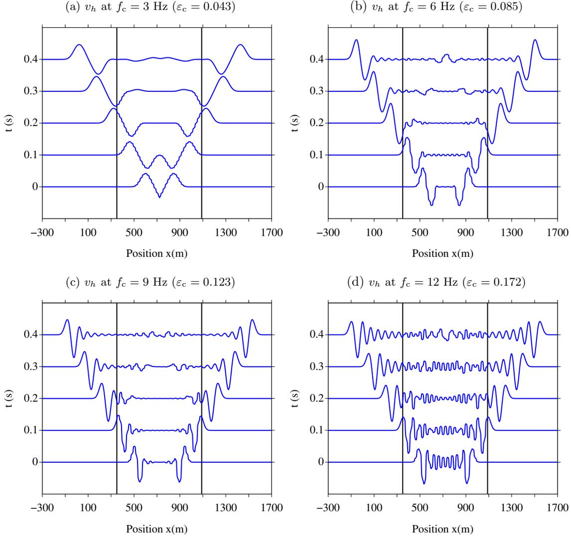
**Figure 8.** Waves emitted in a microstructured slab surrounded by two homogeneous half-spaces: microstructured velocity  $v_h$  for several source frequency and times. For the clarity of the figure, the internal interfaces are not shown.
