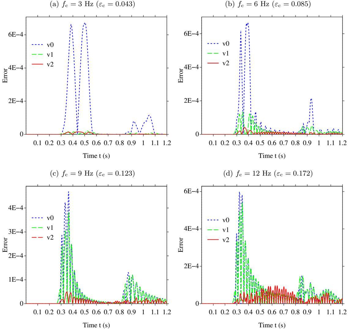
**Figure 11.** Waves emitted in a microstructured slab surrounded by two homogeneous half-spaces. Time evolution of the errors  $|v_n(x_r, t) - v_n(x_r, t)|$  at receiver  $x_r$ , with the orders  $n = 0, 1, 2$ .
