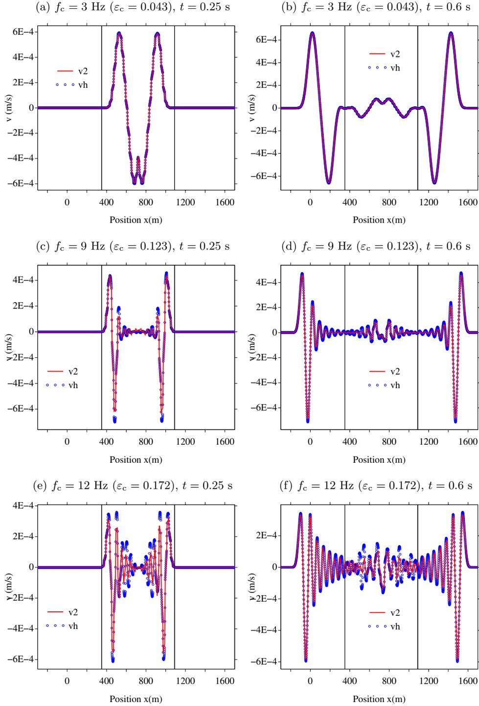
**Figure 9.** Wave emitted by a source point in a heterogeneous slab: comparisons between “total” velocity  $v_2$  (Section 3.4) and the microstructured field  $v_h$  at three central frequencies (rows), represented at  $t = 0.25$  (left column) and  $t = 0.6$  (right column).
