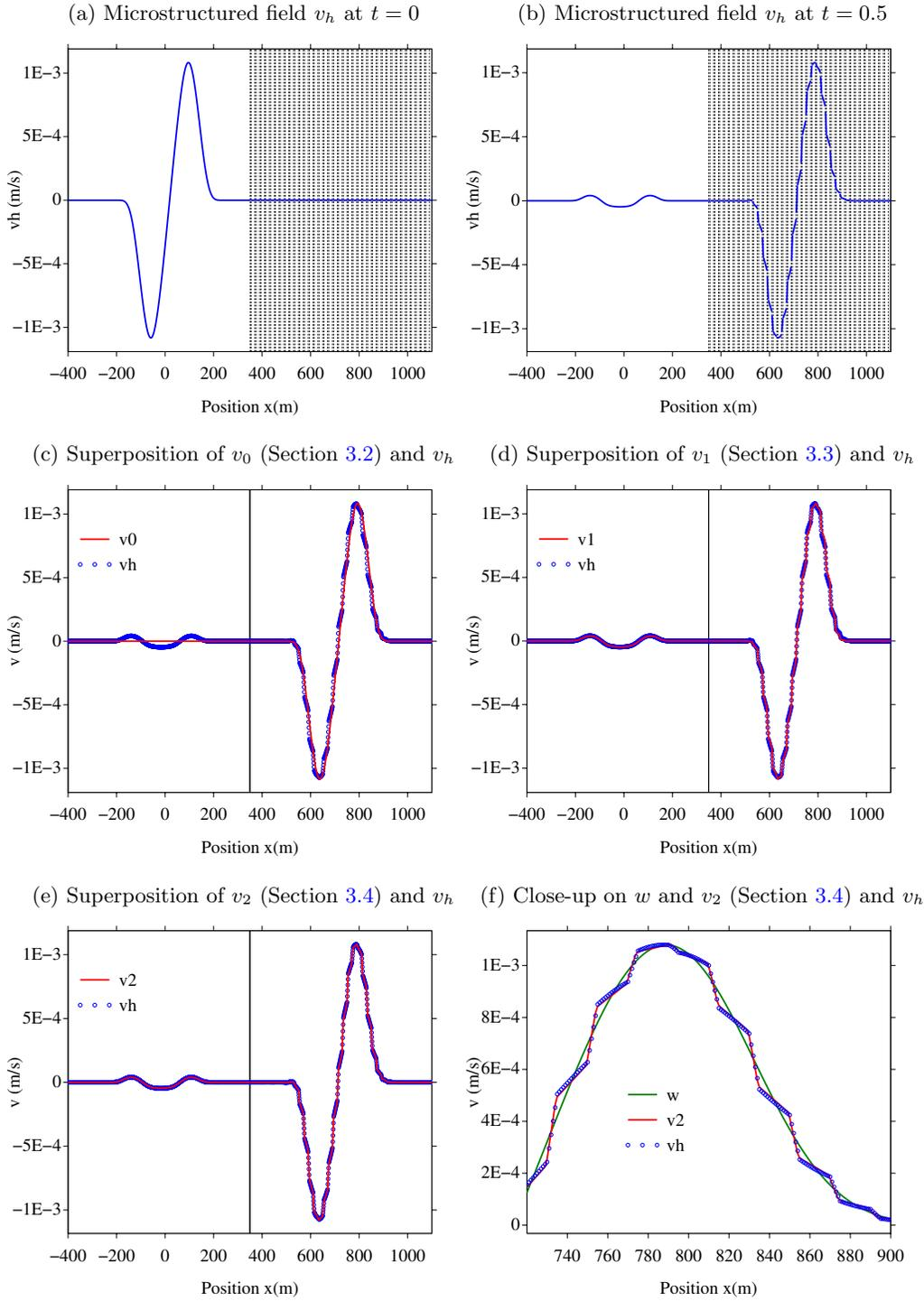
**Figure 3.** Wave in a homogeneous half-space (a-b, left) impacting a microstructured half-space (a-b, right) with impedance matching ( $E_-\rho_- = E_0\rho_0$ ). The central frequency is  $f_c = 3$  Hz ( $\varepsilon_c = 0.043$ ).
