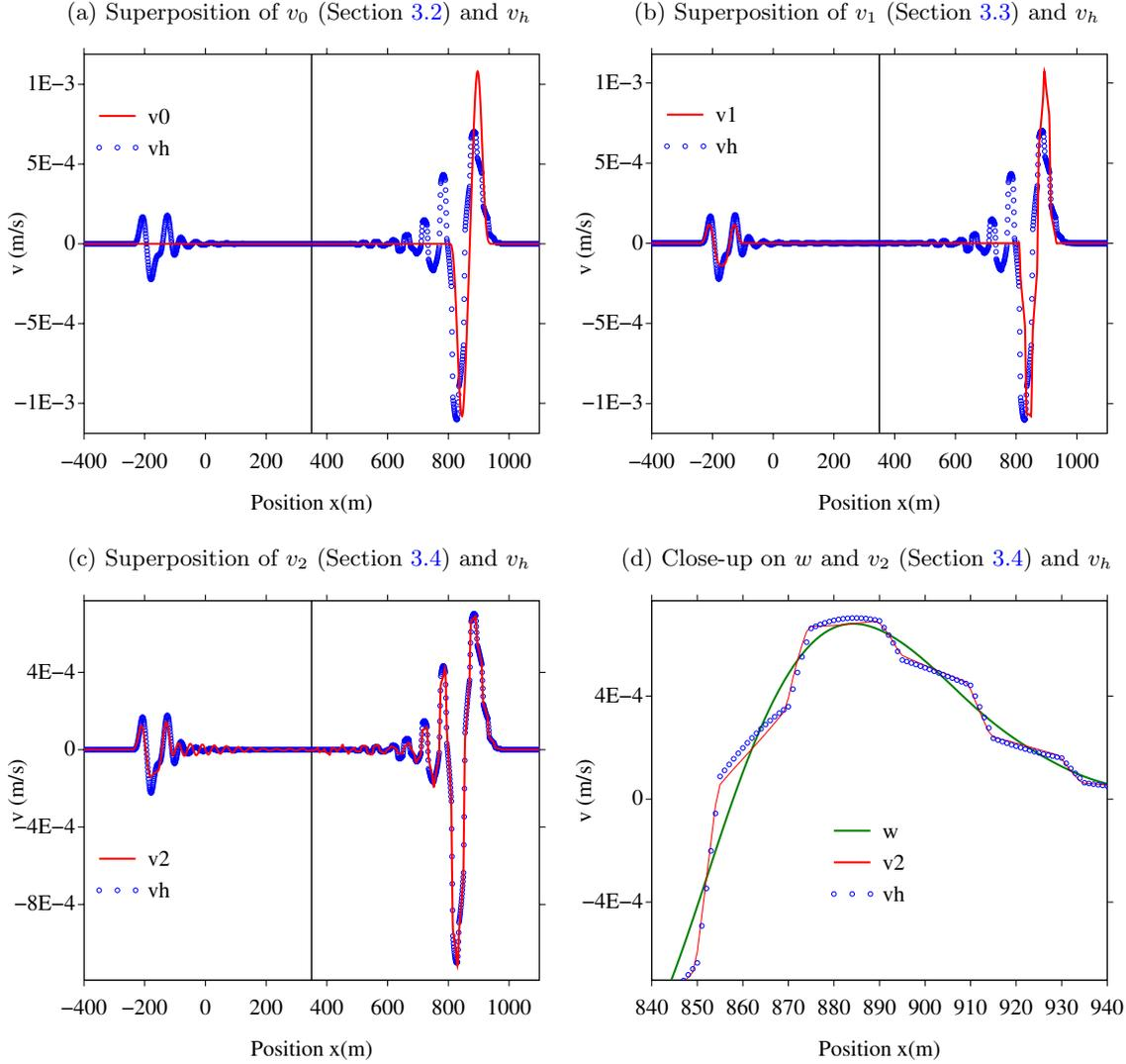
**Figure 4.** Interface between a homogeneous half-space and a microstructured half-space. The central frequency is  $f_c = 9$  Hz ( $\varepsilon_c = 0.123$ ), and time is  $t = 0.5$ .
