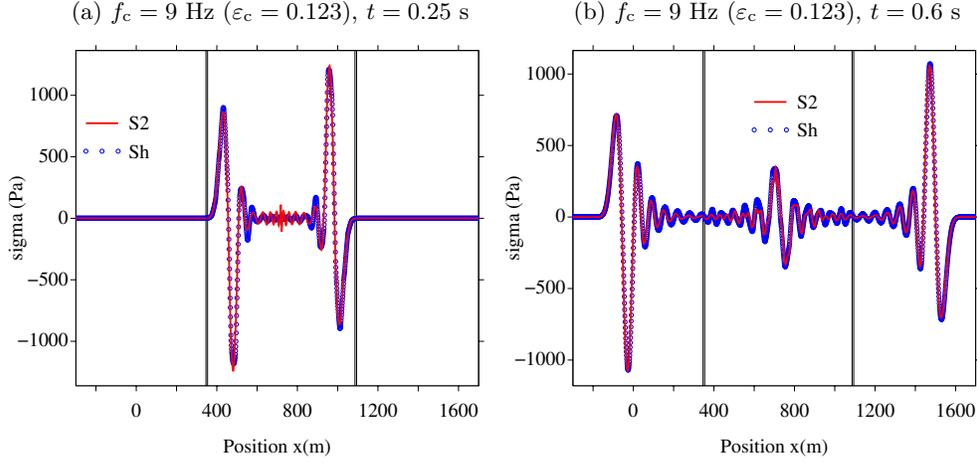
**Figure 10.** Wave emitted by a source point in a heterogeneous slab: comparisons between “total” stress  $\sigma_2$  (Section 3.4) and the microstructured field  $\sigma_h$  at central frequency  $f_c = 9$  Hz (central row of Figure 9), represented at  $t = 0.25$  (a) and  $t = 0.6$  (b).
