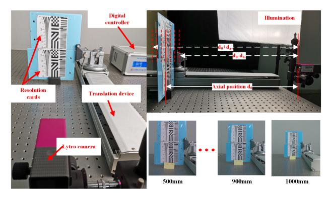
Fig. 9. Experimental setup of refocus precision evaluation for the 1st generation Lytro camera at different axial positions.
