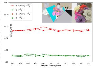
Fig. 8. Validation of the proposed refocus precision model. We show the LPC-SI between images refocused on adjacent planes within and outside the refocus precision limit  $Arp = [d - d(\alpha^{-}), d + d(\alpha^{+})]$  at different axial positions. On the top right, the synthetic scene with ideal camera settings is generated using the Blender light field plugin [24] with the parameters shown in Table II.
