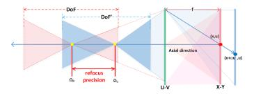
Fig. 3. Difference between light field DoF and refocusing precision. The pink and blue shadowed regions correspond to the definition of traditional DoF. The refocusing precision is defined as the minimum distance Arp between two distinguishable adjacent focal planes in the object space.
