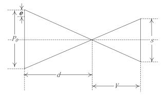
Fig. 13. The relation between  $P_0$ , s and the theoretical shifting limit e of a pin-hole camera with a fixed image plane. Please note that the image plane distance V is a constant. Otherwise, the FoV will vary with different focal lengths f, so that  $P_0$  can not be derived using Equation12 below.
