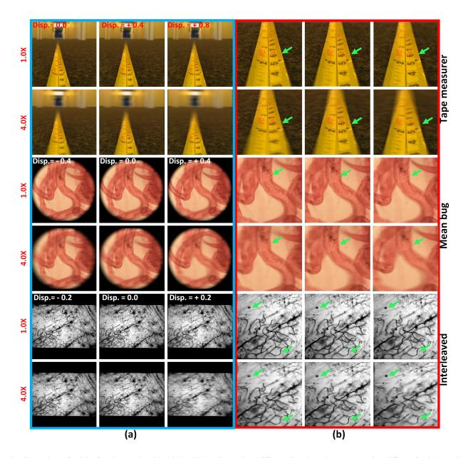
Fig. 12. Comparison of axial refocusing results with 1.0X, 4.0X baselines, where different disparity values correspond to different focal planes in axial direction. (a) Refocused results on same axial focus planes, with 1.0X and 4.0X baselines respectively. (b) Zoomed views, the green arrows are pointing at details on different refocusing planes that are more distinguishable with a 4.0X baseline and less resolvable with the 1.0X baseline.
