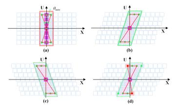
Fig. 2. Differences between original and re-sampled light fields. (a) The original 2D light field, (b) The positive shifting corresponds to a re-sampling of the original light field in (a), in order to move the focus plane closer in the axial direction. (c) The negative shifting is opposite to (b). (d) The shifting leads to a resolvable re-sampling even without sub-pixel interpolation.
