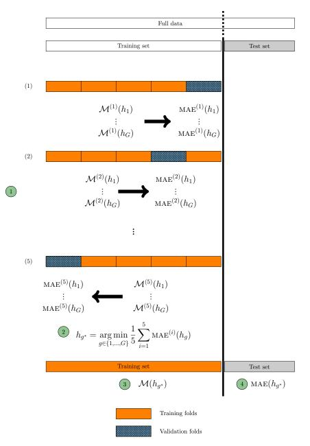
Figure 14: Principle of the automated selection procedure proposed, for a given machine-learning method. The full dataset is split into a train set (in orange) and a test set (in grey). The train set is itself split into a random partition consisting of 5 subsets called folds.
