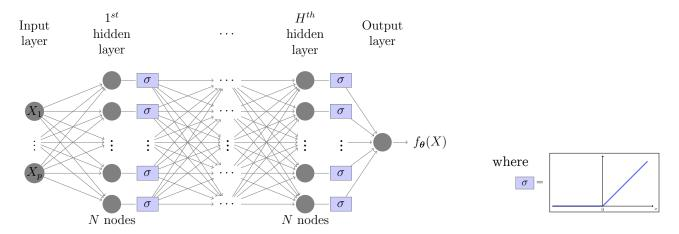
Figure 4: Architecture of the feed-forward networks considered; the  $\sigma$  boxes correspond to the application of the rectified linear unit (ReLU) activation function  $\sigma(x) = \max\{x, 0\}$  depicted on the right.
