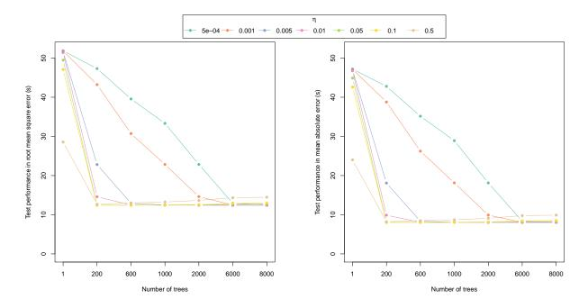
Figure 16: Performance of gradient boosting with regression trees on the test data set for various values of the pair  $(\eta, T)$  of tuning parameters, where  $\eta$  is the shrinkage parameter and T is the number of trees. The left picture measures performance in RMSE and the right picture does so in MAE.
