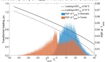
Figure 16: Black lines: transformer loadings corresponding to HST<sub>1%</sub> .Orange and blue bars: PDF of T<sub>amb</sub> in Tomsk and in Grenoble based on 34-years history
