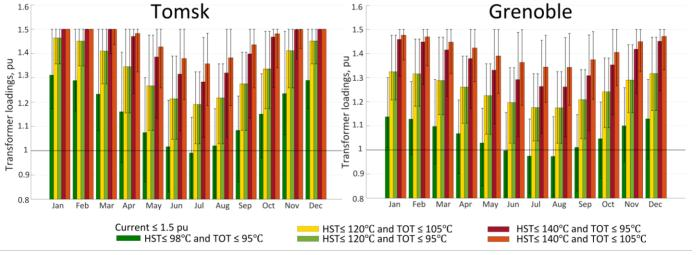
Figure 12: Mean DTR with maximum and minimum deviations in each month
