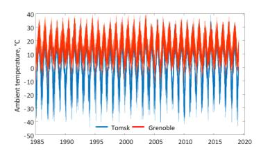
Figure 9: Hourly T<sub>amb</sub> from 1985 to 2019 in Tomsk and Grenoble
