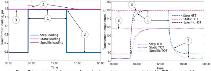
Figure 5: Interrelations between transformer loading and temperatures, calculated by IEC thermal model
