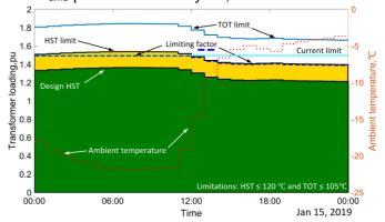
Figure 8: Feasible region limited by current and HST From Fig. 8 we see that once  $T_{amb}$  crosses the critical  $T_{amb}$  = -17 °C (Fig.1), the limiting factor shifts from current = 1.5 pu to HST limit = 120 °C.
