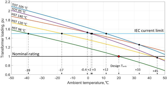
Figure 1: Transformer loadings equal to HST and TOT limits as a function of Tamb
