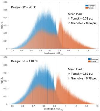
Figure 17: Loadings which can be used for compensation of accelerated LoL (based on historical T<sub>amb</sub>)
