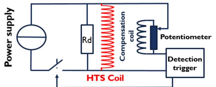
**Figure 1.** Electrical circuit to test our superconducting coils.
