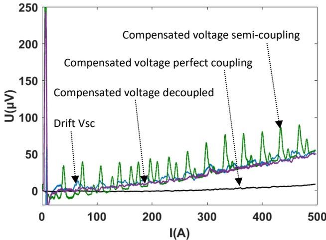
**Figure 25.** Compensated experimental voltages compared to the inductive drift from the REBCO pancake for the second and following current ramps up to 500 A. The compensated voltage of the perfectly coupled mutual is in black. The compensated voltage of the semi-coupled mutual in green as well as the compensated voltage of the decoupled mutual in purple merge perfectly with the REBCO coil voltage drift in light blue.
