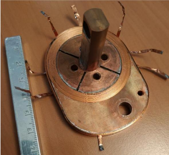
**Figure 4.** Single insulated REBCO pancake with a co-wound pick-up coil.
