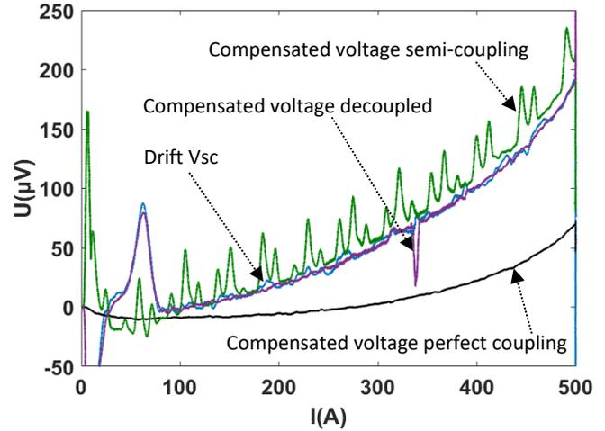
**Figure 23.** Compensated experimental voltages compared to the inductive drift from the REBCO pancake for the first current ramp up to 500 A. The compensated voltage of the perfectly coupled mutual is in black. The compensated voltage of the semi-coupled mutual in green as well as the compensated voltage of the decoupled mutual in purple merge perfectly with the REBCO coil voltage drift in light blue.
