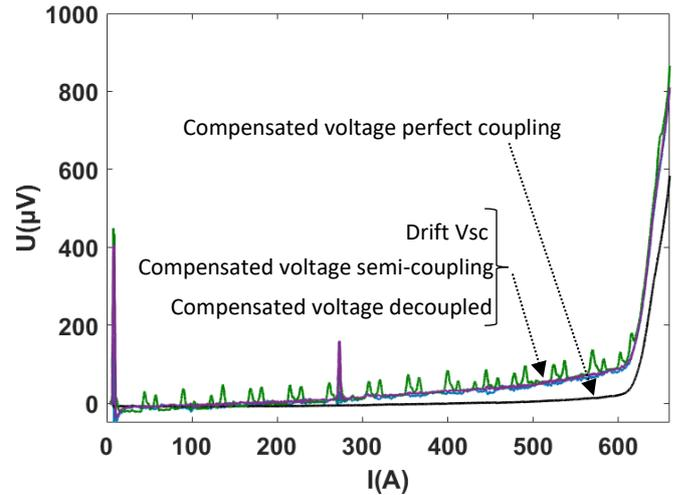
**Figure 30.** Compensated experimental voltages compared to the inductive drift from the REBCO pancake up to a runaway. The compensated voltage of the perfectly coupled mutual is in black. The compensated voltage of the semi-coupled mutual in green as well as the compensated voltage of the decoupled mutual in purple merge perfectly with the REBCO coil voltage drift in light blue.
