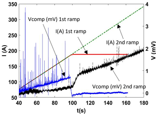
**Figure 3.** Dependence of the first and second (and following) current ramps on inductive voltage. The first current ramp in red and its compensated voltage in blue. The second current ramp in green dotted line and its compensated voltage in black.
