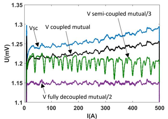
**Figure 24.** Voltages from the REBCO pancake ( $V_{sc}$ , light blue) and the 3 pick-up coils ( $V$  coupled mutual in black,  $V$  semi-coupled mutual/3 in green and  $V$  fully decoupled mutual/2 in purple) for the second and the following current ramp up to 500 A.
