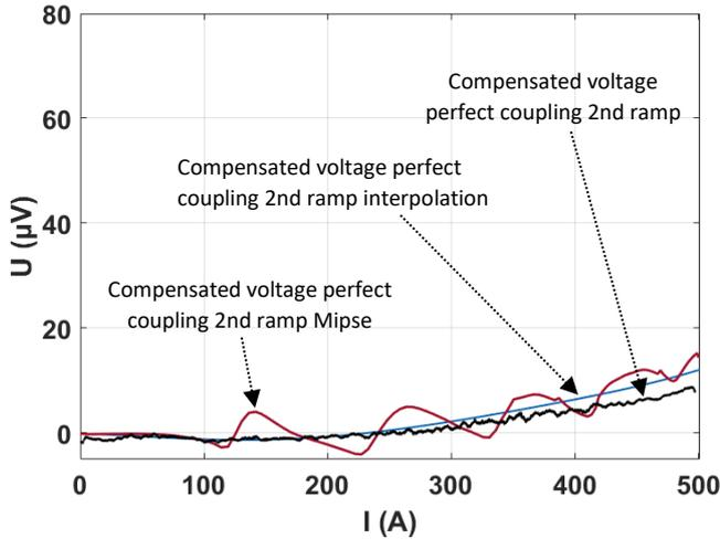
**Figure 28.** Compensated experimental voltage with a “perfect” coupling for the second current ramp up to 500 A compared to the modelling results. Experimental curve in black, Mipse curve in red and the interpolation in blue.
