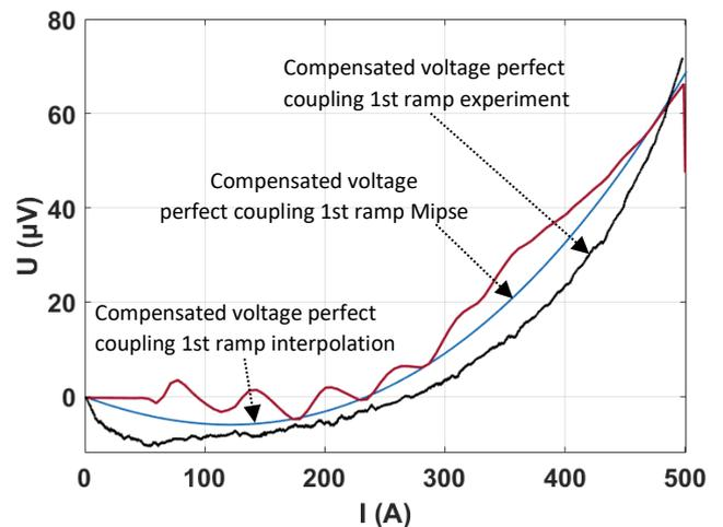
**Figure 27.** Compensated experimental voltage with the “perfect” coupling for the first current ramp up to 500 A compared to the modelling results. Experimental curve in black, Mipse curve in red and the interpolation in blue.
