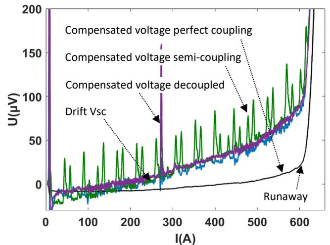
**Figure 31.** Zoom on compensated experimental voltages compared to the inductive drift from the REBCO pancake up to a runaway. The compensated voltage of the perfectly coupled mutual is in black. The compensated voltage of the semi-coupled mutual in green as well as the compensated voltage of the decoupled mutual in purple merge perfectly with the REBCO coil voltage drift in light blue.
