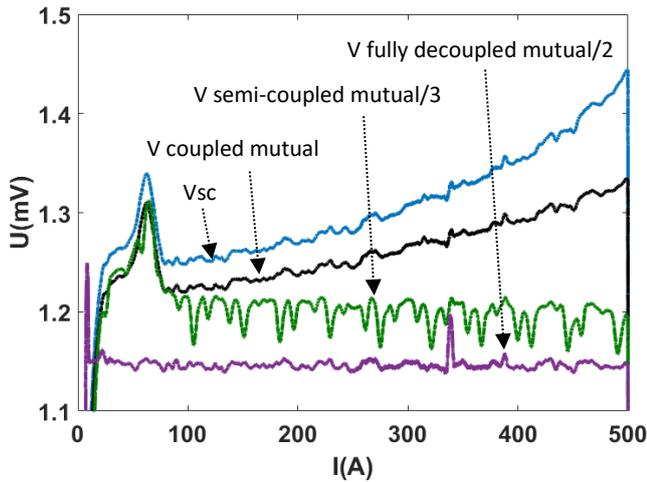
**Figure 22.** Voltages from the REBCO pancake ( $V_{sc}$ , light blue) and the 3 pick-up coils ( $V$  coupled mutual in black,  $V$  semi-coupled mutual/3 in green and  $V$  fully decoupled mutual/2 in purple) for the first current ramp up to 500 A.
