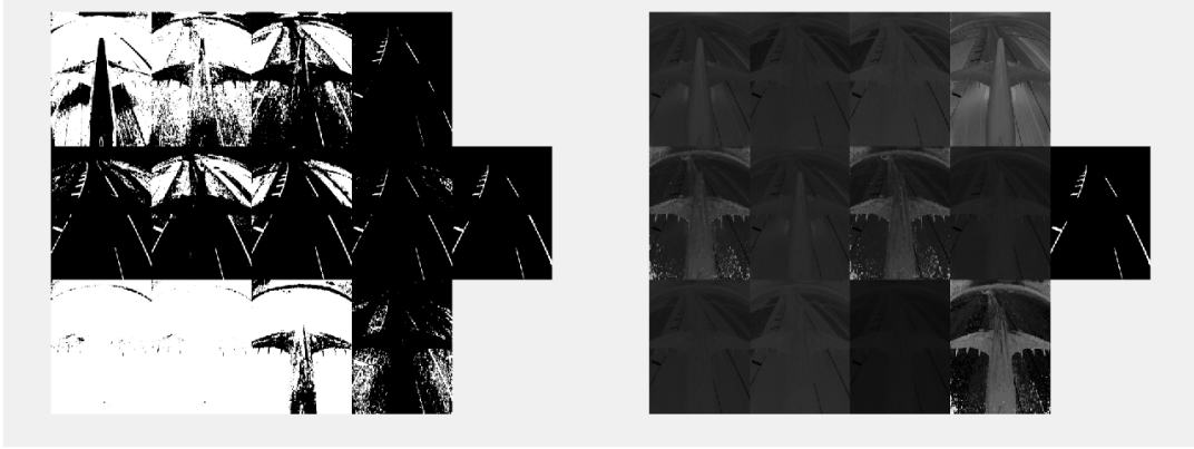
Figure 4: Example of Binary (left) and Distance (right) maps for fin camera images. First line: \Delta E^*_{ab} , \Delta E_{AB} , \Delta E_B , \Delta E^*_{00} . Second line: \Delta E_{LCH} , \Delta C_{LCH} , \Delta E_{CH} , \Delta E^*_{CMC} , ground truth. Third line: \Delta E_{CbCr} , \Delta E_{Cb} , \Delta E_{IQ} , \Delta E_H (HSV/HSL).
