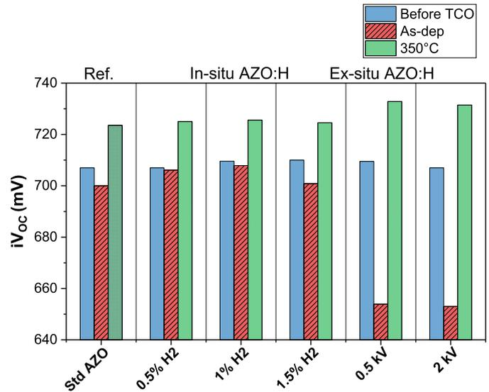
Fig. 7. Variation of  $iV_{\text{OC}}$  of symmetrical samples featuring poly-Si n<sup>+</sup>/SiO<sub>x</sub> with TCO layers composition and at different process steps.
