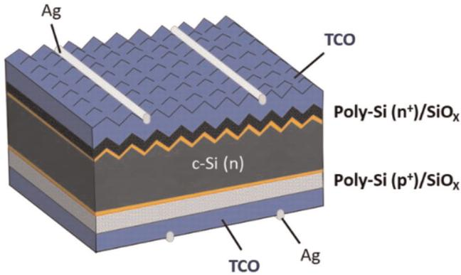
**Fig. 1.** c-Si solar cell structure in rear emitter configuration with double side passivated contacts elaborated by high (poly-Si/SiO<sub>x</sub>) temperature route.
