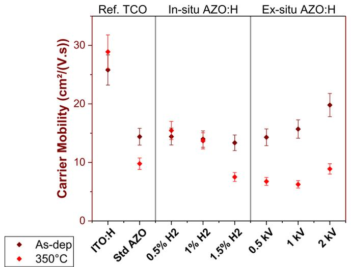
**Fig. 4.** Variation of charge carrier mobility with the TCO composition and the annealing at 350 °C.
