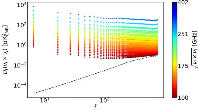
**Fig. 1.** Mean value over the  $N_{\text{sim}}$  simulations of the  $B$ -mode angular power spectra  $\mathcal{D}_\ell(v_i \times v_j)$  for the d1c simulation type, with  $r_{\text{sim}} = 0$ . The color bar spans all the  $N_{\text{cross}}$  spectra  $\mathcal{D}_\ell(v_i \times v_j)$ , associated to their reduced cross-frequency  $\nu_{\text{red.}} = \sqrt{v_i v_j}$ , from 100 GHz (dark red) to 402 GHz (dark blue). The input CMB lensing power spectrum is shown as a black dashed line.
