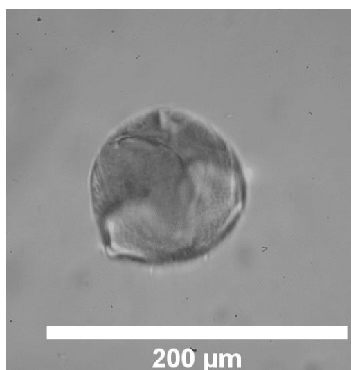
FIG. S5. Frame taken from movie 'FigS5_Mesogel_shrinking_3Cpmin_x20.mp4' – available as an independent supplementary material file – showing the shrinkage of a PNIPAM mesogel suspended in a commercial Ludox suspension ( \phi = 0.350 ) and heated at \dot{T}_{\text{up}} = 3^\circ\text{C}/\text{min} . Magnification: \times 20 . Field of view dimensions: 234 \mu\text{m} \times 244 \mu\text{m} . Exposure time: 20 ms. Video recorded with a high-speed camera at 24 fps and played at recording speed. Multimedia view.
