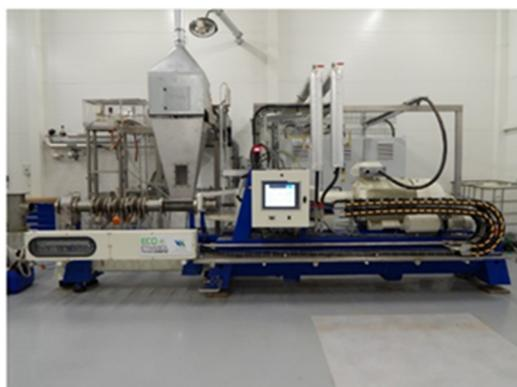
**Figure 1.** Extruder Clextral Evolum EV 53 for polyphenol extrusion-extraction.
