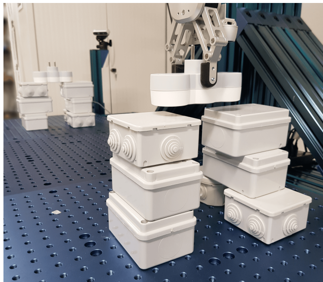
Fig. 1. Example result of our approach. A UR5 manipulator assembles a configuration of known primitives (right - foreground). The configuration is specified by a single photograph of the assembly (camera on the left - background).
