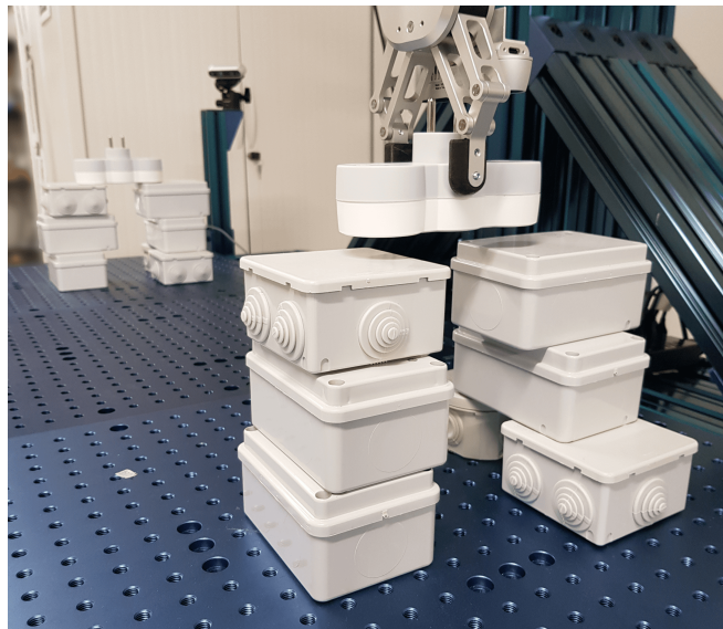
Fig. 1. Example result of our approach. A UR5 manipulator assembles a configuration of known primitives (right - foreground). The configuration is specified by a single photograph of the assembly (left - background).
