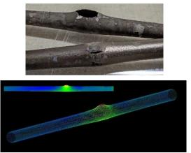
Fig. 8. Post-test examination results. Top: final aspect of burst dummy rods (pre-oxidised Zircaloy cladding,  $Al_2O_3$  pellets, after several ramps). Bottom: 3D post-test laser metrology.
