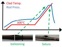
Fig. 1. LOCA sequence and clad expected behaviour.
