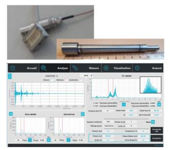
Fig. 4. Ultrasonic sensor. Top left: the sensor and its connector. Top right: the plenum cavity on which the sensor is stuck. Bottom: the associated HORTUS software (example of measurement on a cavity filled with a 10%Xe in He standard gas mixture at 55bar and room temperature).
