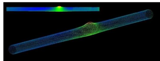
Fig. 8. Post-test examination results. Top: final aspect of burst dummy rods (pre-oxidised Zircaloy cladding, Al<sub>2</sub>O<sub>3</sub> pellets, after several ramps). Bottom: 3D post-test laser metrology.
