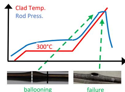
Fig. 1. LOCA sequence and clad expected behaviour.
