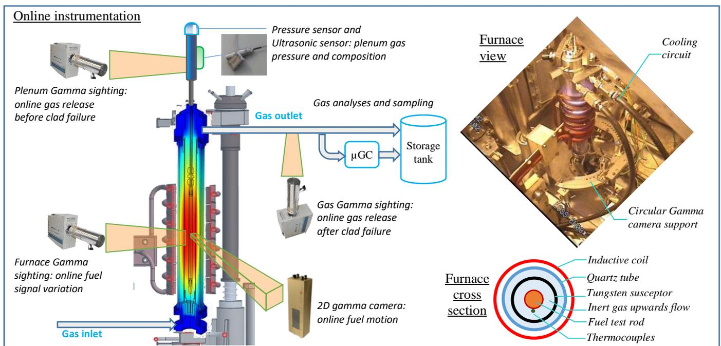
Fig. 2. VINON-LOCA online instrumentation, furnace view and furnace cross section
