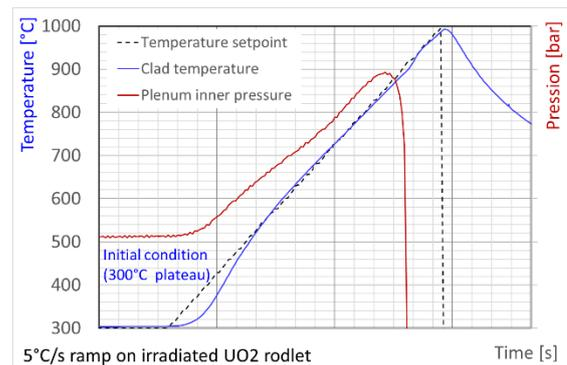
Fig. 7. Clad temperature and rod inner pressure recordings during the first test on irradiated UO<sub>2</sub>.
