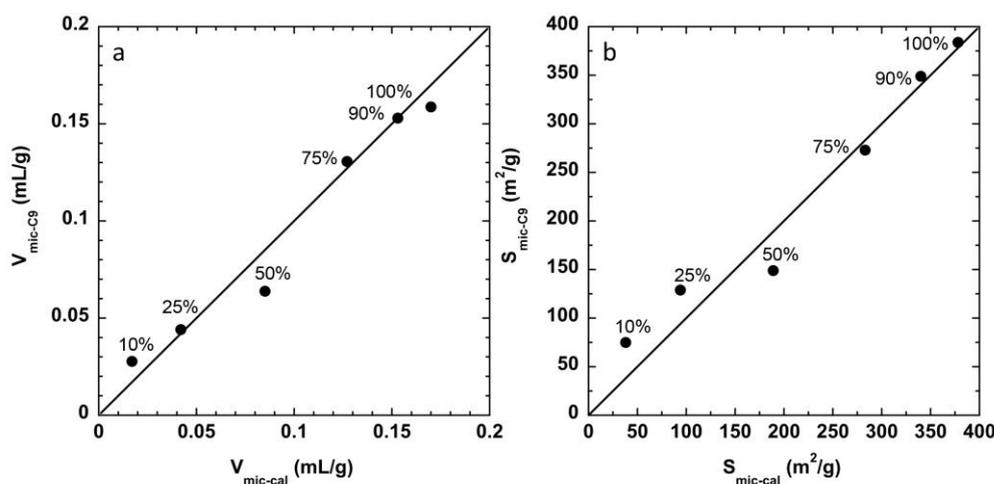
**Figure 7** (left) Micropore volumes (taken at  $p/p_0 = 0.42$ ) and (right) micropore surface areas determined from the nitrogen isotherms recorded for the mechanical mixtures of ZSM-5 (Si/Al = 40) and Si-MCM-41(C16) pre-adsorbed with *n*-nonane. The values were compared with the predicted calculated values determined based on the weight percentage of each material.
