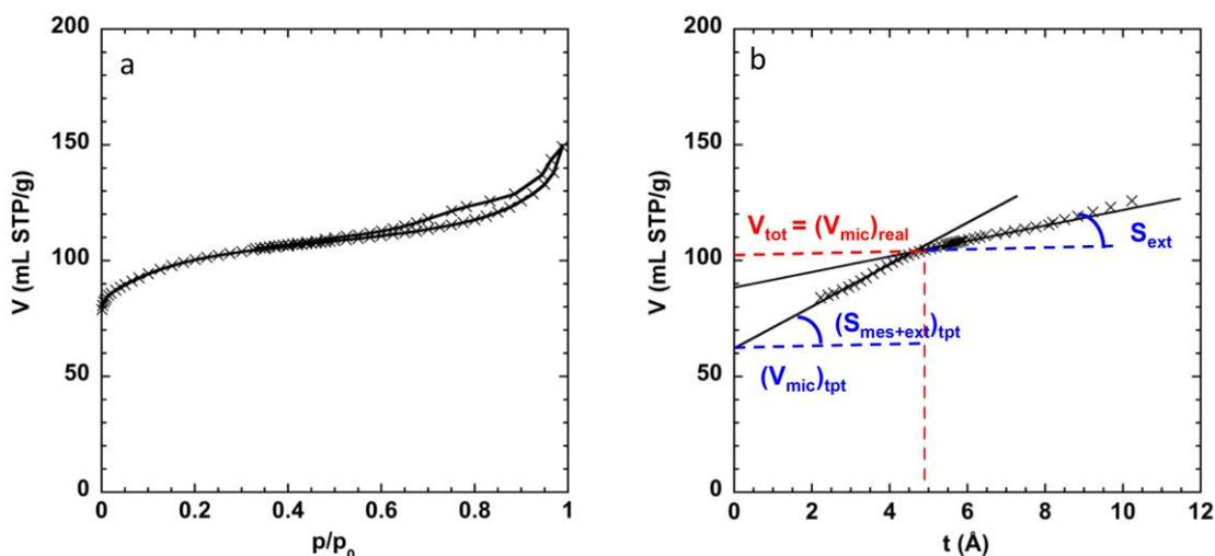
**Figure 2** (a)  $N_2$  sorption isotherm at 77 K of ZSM-5 (Si/Al = 15) and (b) corresponding  $t$ -plot.
