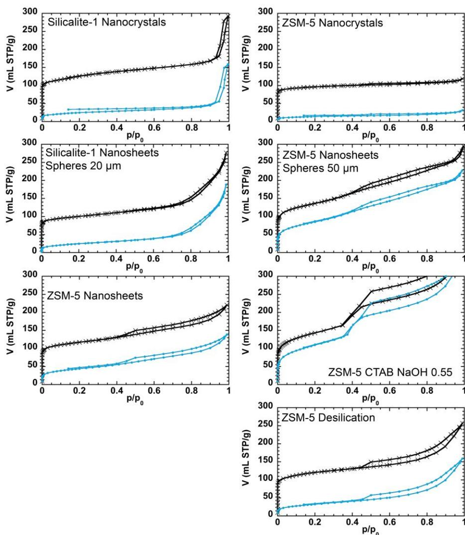
**Figure 9** N<sub>2</sub> sorption isotherms recorded at 77 K for different hierarchical MFI-type zeolites. The isotherms were recorded (crosses) before and (circles) after *n*-nonane adsorption and outgassing processes.
