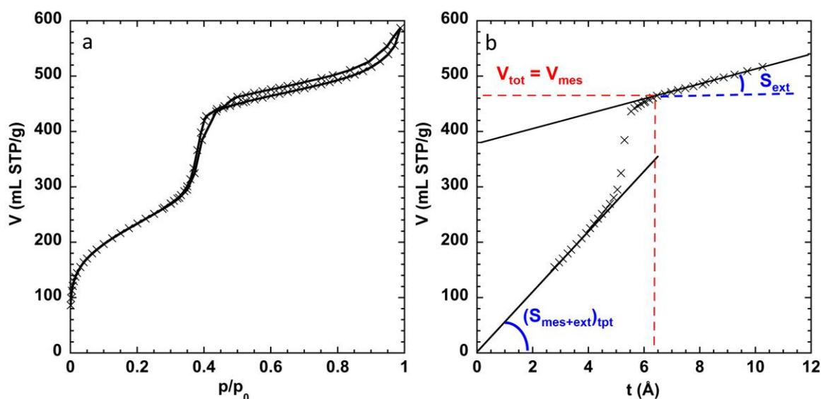
**Figure 1** (a) N<sub>2</sub> sorption isotherm recorded at 77 K for Al-MCM-41(C18) and (b) corresponding  $t$ -plot.
