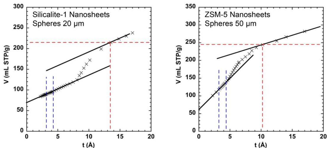
**Figure 10** Analysis of  $t$ -plots generated for hierarchical ZSM-5 systems. Range of  $t$  for the first fit at low  $t$  (dashed blue lines) and the starting point of  $t$  (vertical red dashed line) for the second fit at high  $t$  correspond to (horizontal red dashed line) the “total” pore volume (micropore + mesopore volumes).
