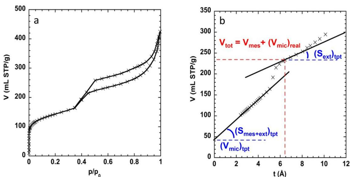
**Figure 3** (a)  $N_2$  sorption isotherm recorded at 77 K for hierarchical ZSM-5 (Si/Al = 15) prepared following the micelle-templating (NaOH/Si = 0.55) method and (b) corresponding  $t$ -plot.
