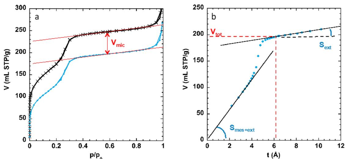
**Figure 5** (left) N<sub>2</sub> sorption isotherms recorded at 77 K for the mechanical mixture prepared with 50 wt.% of ZSM-5 (Si/Al = 40) and 50 wt.% of Si-MCM-41(C16) in the presence (blue points) and absence (crosses) of pre-adsorbed *n*-nonane. (right) The Corresponding *t*-plot obtained following the pre-adsorption of *n*-nonane showing the absence of microporosity.
