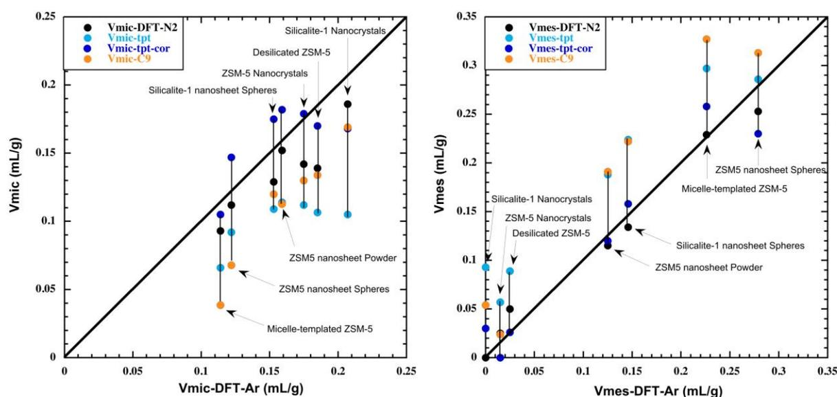
**Figure 11** Comparison of (left) micropore and (right) mesopore volumes obtained by the different methods:  $t$ -plot, corrected  $t$ -plot, pre-adsorption of  $n$ -nonane followed by N<sub>2</sub> adsorption at 77 K, NLDFT based on the N<sub>2</sub> isotherm at 77 K (comparison was made with the volumes determined using the NLDFT method based on the Ar isotherm recorded at 87 K) for the different hierarchical MFI-type zeolites.
