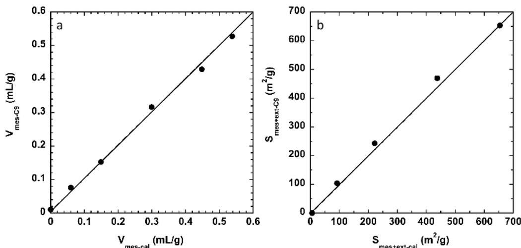
**Figure 6** (a) Mesopore volumes and (b) mesopore surface areas recorded post *n*-nonane pre-adsorption for the mechanical mixture of ZSM-5 (Si/Al = 40) and Si-MCM-41(C16). The values are compared with the predicted calculated values for each material.
