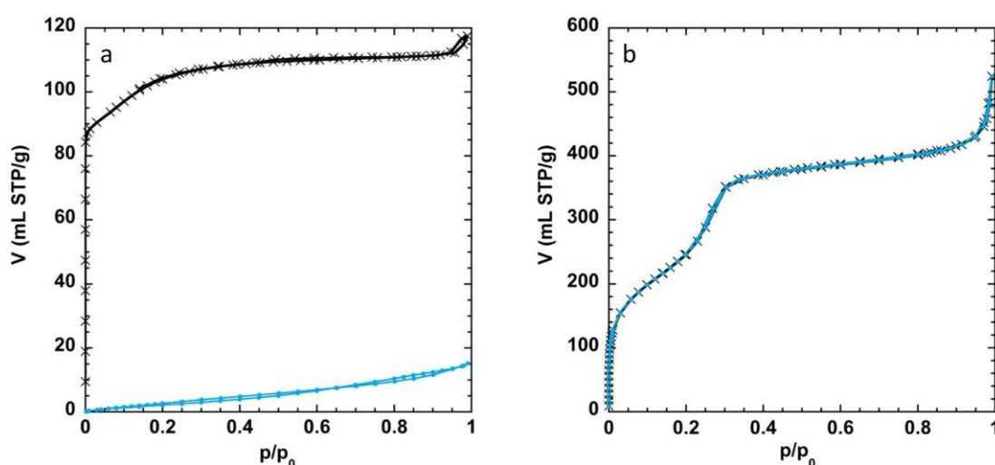
**Figure 4** N<sub>2</sub> sorption isotherms recorded at 77 K for (a) ZSM-5 (Si/Al = 40) and (b) Si-MCM-41(C16) in the presence (blue points) and absence (black crosses) of pre-adsorbed *n*-nonane.
