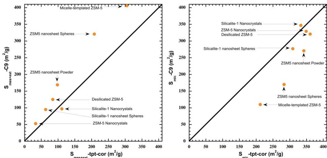
**Figure 12** (left) Mesopore plus external surface areas and (right) micropore surface areas determined following the *n*-nonane pre-adsorption method. The results were compared with the results obtained using the corrected *t*-plot method for hierarchical MFI-type zeolites. Error is  $\pm 10$  m<sup>2</sup>/g for both methods.
