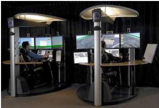
Figure 3. Test bench for UAVs command and control system (Copyright © 1999-2011 by Aero-News Network, Inc. All rights reserved)
