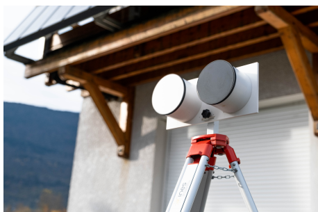
Figure 17: SENS probe used to measure the equivalent outdoor surface temperature of the building
