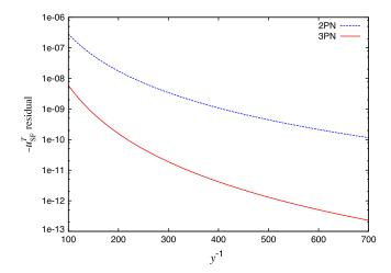
FIG. 3 (color online). Numerically derived residuals, i.e. after removal of the 2PN and 3PN self-force contributions to  $u_{SF}^T$ , plotted as a function of the gauge invariant variable  $y^{-1}$ . Compare with scales in Fig. 2. Note that  $y^{-1}$  is equal to  $R_{\Omega}/m_2$ , an invariant measure of the orbital radius, scaled by the black hole mass  $m_2$  [cf. Eq. (2.16)].
