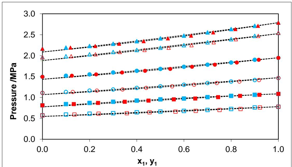
Figure 4a: Vapor liquid Equilibrium data for the nitrogen (1) + carbon monoxide (2) binary system from 100 ( $\square$ ), 105 ( $\blacksquare$ ), 110 ( $\circ$ ), 115 ( $\bullet$ ), 120 ( $\Delta$ ) and 122 K ( $\blacktriangle$ ), in blue: bubble point, in red: dew point. Experimental data from Torocheshnikov [8]. Dashed line: Peng Robinson EoS.
