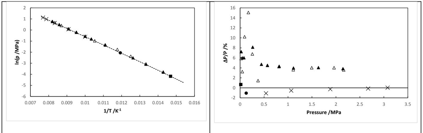
**Figure 5. A: Vapor pressure of carbon monoxide as a function of temperature, experimental and calculated values (solid line: prediction from DIPPR's correlation (■): Duncan and Staveley, (Δ): Torocheshnikov, (●): Sprow and Prausnitz, (▲): Yushkevich and Torochechnikov, (×): this work.). B: Relative deviations of CO vapor pressure from the different authors in comparison to the DIPPR correlation's prediction.**
