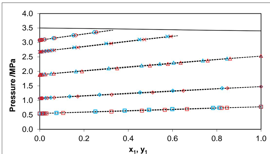
**Figure 1: Phase boundaries of the binary system nitrogen (1) + carbon monoxide (2) at 100.2 (□), 110.07 (◇), 120.05 (△), 127.07 (×) and 130.07 K (○), experimental and calculated values (symbols this work (in blue: bubble point, in red: dew point), dashed line: PR EoS, solid line: mixture critical line).**
