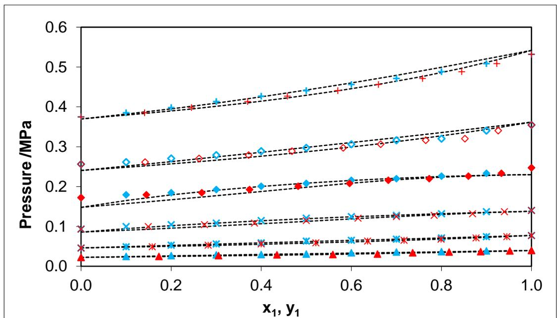
Figure 4b: Vapor liquid Equilibrium data for the nitrogen (1) + carbon monoxide (2) binary system from 70 ( $\blacktriangle$ ), 75 ( $*$ ), 80 ( $\times$ ), 85 ( $\blacklozenge$ ), 90 ( $\diamond$ ) and 95 K ( $+$ ), in blue: bubble point, in red: dew point. Experimental data from Torocheshnikov [8]. Dashed line: Peng Robinson EoS.
