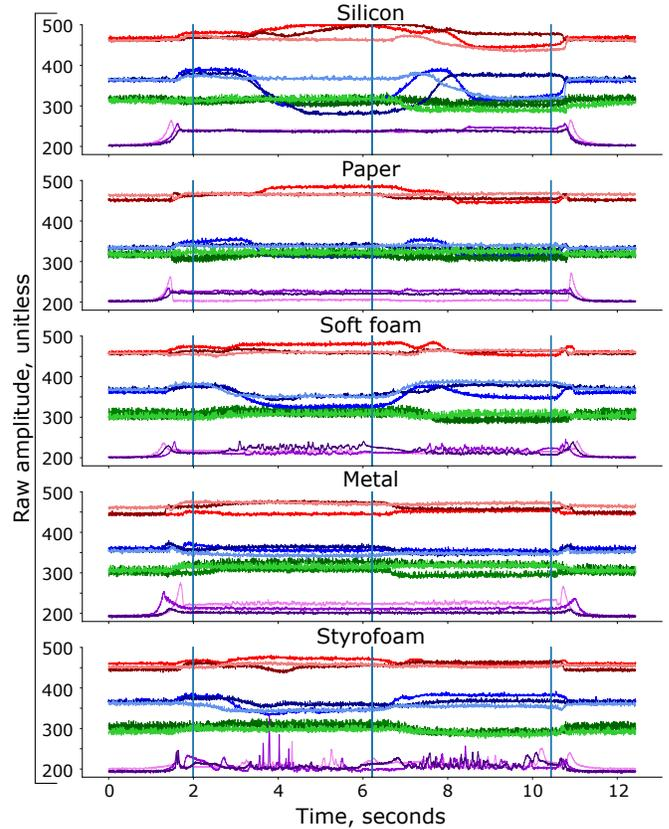
Fig. 5. The raw output of the tactile sensor for different materials. Reds: D1, blues: D2, greens: D3, purples: P. Leftmost vertical blue line represents the start of the sliding motion; the middle vertical blue line represents the reverse in slide direction; the rightmost vertical blue line represents the end of the slide.
