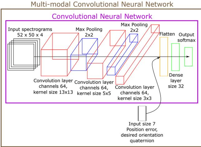
Fig. 4. Convolutional neural network (CNN) and multi-modal CNN classifiers. Classifiers are similar except for the additional input layer that contains the robot’s end-effector position error and scan orientation quaternion.
