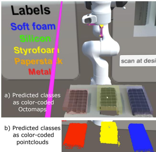
Fig. 8. Classification results visualized in Virtual Reality interface: a) classification results as color-coded Octomaps overlaid on corresponding objects; b) classification results as static color-coded segmented pointcloud clones.
