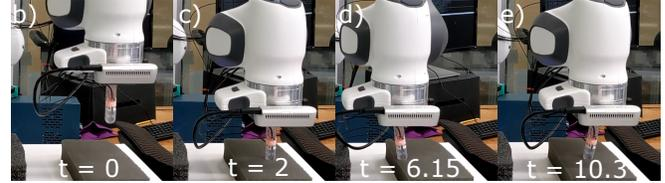
Fig. 2. a) The operator manually sets the scan reference pose: the pose of the 3D blue axis mesh is used as a reference of scan location with the second reference at 56.5mm offset. b) the robot approaches to the scan start position at  $t = 0$ ; c) the slide begins at  $t = 2$ ; d) the slide direction reverses at  $t = 6.15$ ; e) the slide is finished at  $t = 10.3$ .
