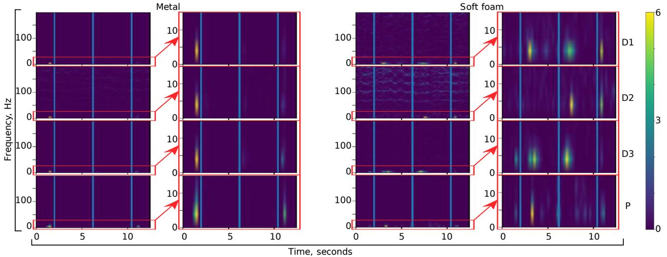
Fig. 6. Sample spectrograms (not normalized) for metal and soft foam. There are large spikes in 0-15Hz frequency range for both materials (arrows indicate zoom-in regions) and smaller spikes in high frequency for softer/rougher soft foam.
