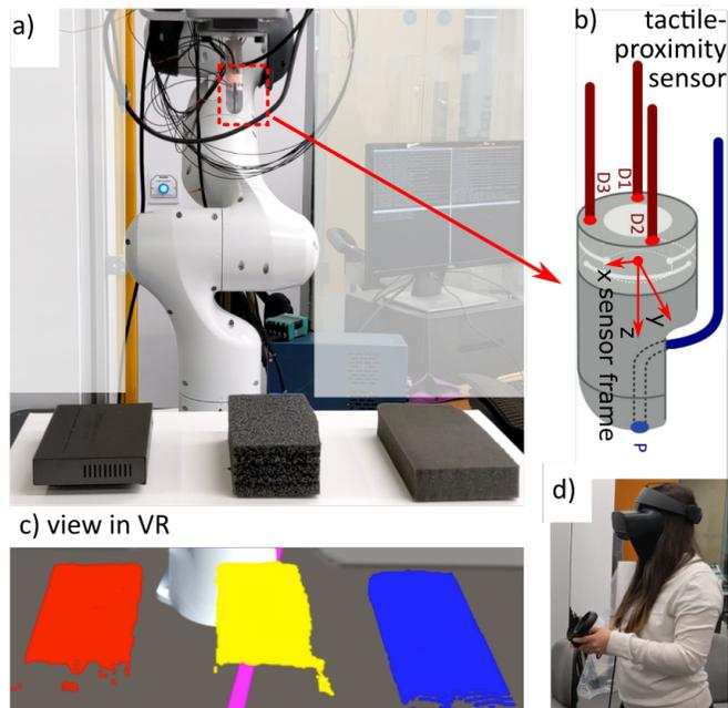
Fig. 1. Overview of the system. **a)** a remotely operated robotic-manipulator with a tactile sensor **(b)** is commanded by a human-operator **(d)** to explore the surfaces of different objects. Material classification results are used to visualise the objects differently in the VR reconstruction **(c)**.
