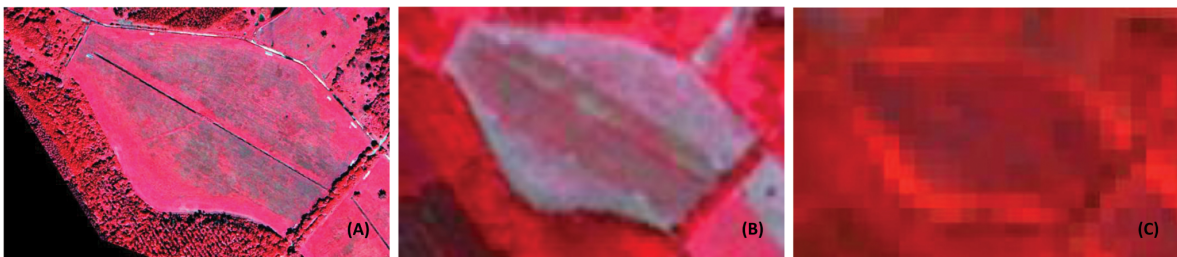
Figure 2.11: Spatial resolution comparison (false color composite: R = NIR, G = RED, B = GREEN) among QuickBird (A; res. spat = 0.65m), RapidEye (B; res. spat = 5m) and Landsat-8 (C; res. spat = 30m) covering a managed natural grassland conservation site in the west of Berlin, Germany (Courtesy: Dr Michael Förster) [ACD + 16]
