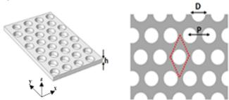
Figure 1. 3D and top-view representation of the polymer photonic membrane. The red dotted lines represent the elementary unit cell.
