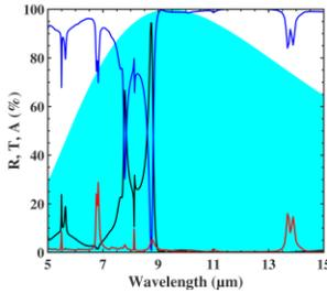
Figure 3. Reflection (black), transmission (blue) and absorption (red) spectra for the structured PE membrane with the geometrical parameters:  $h = 5.1 \mu\text{m}$ ,  $D = 7.1 \mu\text{m}$  and  $P = 9 \mu\text{m}$ .
