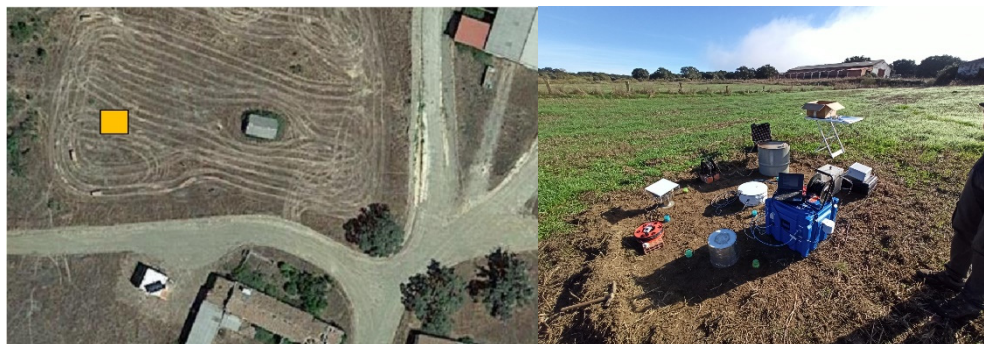
Figure 2. Aerial view and picture of the devices placed in the high radon flux area. The yellow rectangle indicates the testing area.
