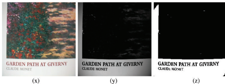
Figure 4: (x) Original image “Contrast = 336.098, Energy = 0.00111243” (y) Modified image “ \gamma = 5.5 ” (z) Binarized image “ T = 0.292969 ”
