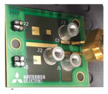
Fig. 8: Close-up on the PCB under test (Dimensions: 35mm\*45mm) and the tip of the Keysight 42941A probe placed across the decoupling capacitor footprint to measure the power loop impedance (decoupling capacitors not mounted).
