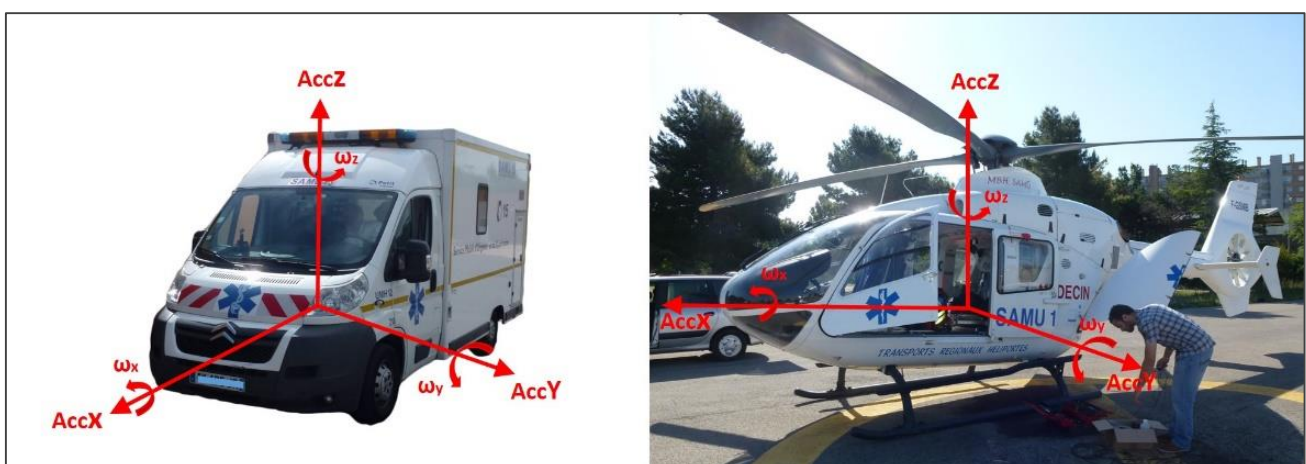
Figure 2. Coordinate system used for vehicles (ambulance and helicopter).
