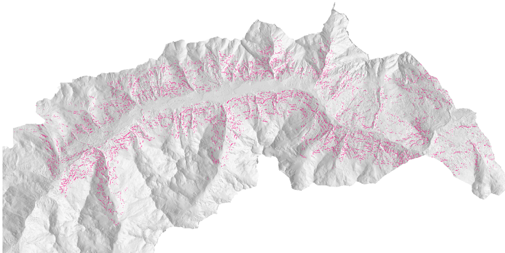
Figure 134: snow avalanches potential release areas under forest canopy map obtained with Avalfor LIN , for the Austrian case study.
