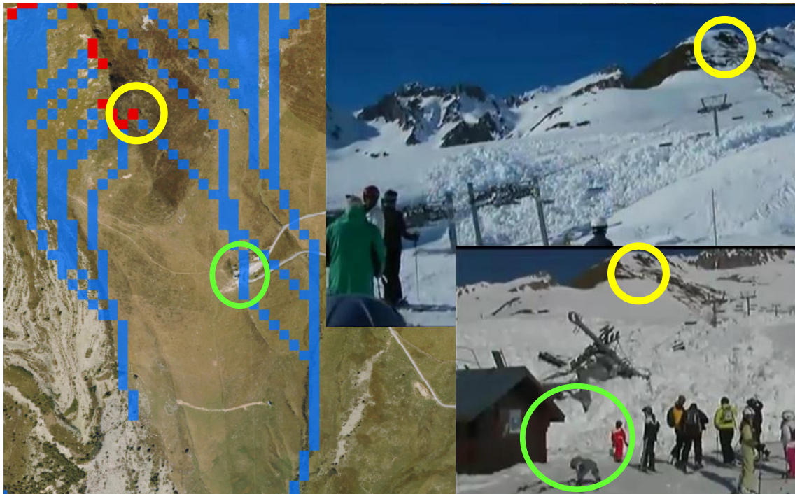
Figure 132: An example of validation of the results obtained with Avalfor LIN using a real event which had occurred in another region than the one used for the calibration of the French ( \alpha, \beta ) model. In red the release are determined with Avalfor LIN , in blue the travel path determined with Avalfor LIN , in the circles the real zones (yellow = release area, green = stopping point).
