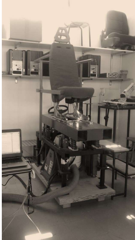
Figure 3: Picture of the test bench and helicopter seat used for the experiment on vertical vibrations.
