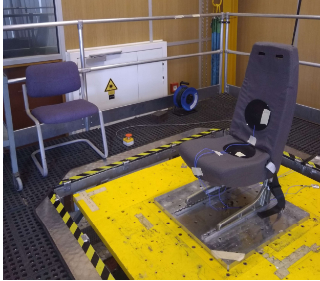
Figure 2: Picture of the Cube, in yellow, on which is mounted a helicopter seat equipped with two pad accelerometers.
