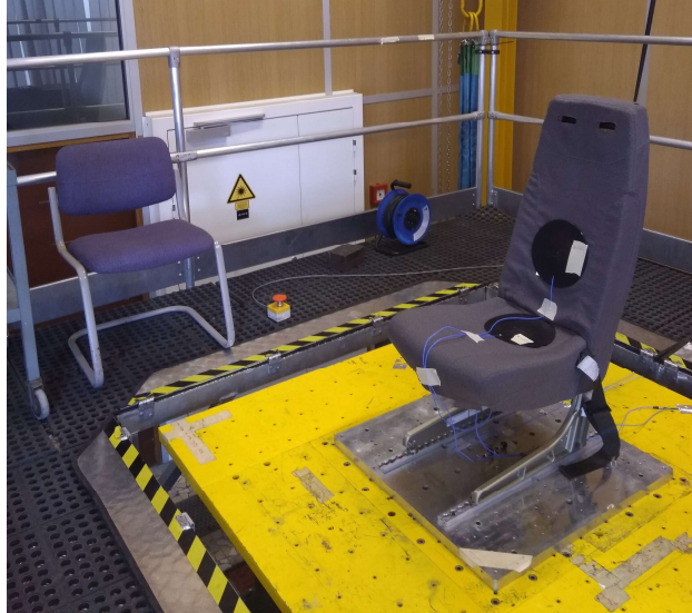
Figure 2: Picture of the Cube, in yellow, on which is mounted a helicopter seat equipped with two pad accelerometers.
