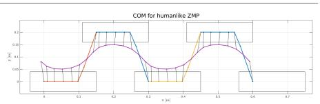
Fig. 7: CoM trajectory (purple) corresponding to a human-like evolution of the ZMP (multicolor).
