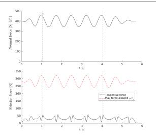
Fig. 13:  $F_z$  Normal (top plot) and  $||F_x + F_y||$  tangential (bottom) components of the reaction force  $F_0$ . The red dashed line represents the maximum acceptable tangential force without risk of slipping.
