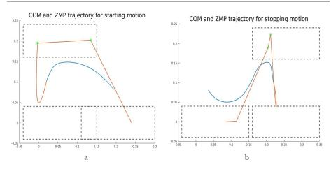
Fig. 11: Imposed ZMP trajectory (orange) and horizontal position of the corresponding CoM (blue) during the starting (a) and the stopping motions (b). The dashed rectangles represent the outlines of the feet on the ground.
