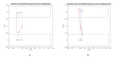
Fig. 12: Evolution of the local ZMP (blue) for each foot respectively during the first and last DS phases of the starting (a) and stopping (b) motions. The dashed lines show the distribution of the global ZMP and the alignment at all times between the two local ZMPs and the global ZMP (red).
