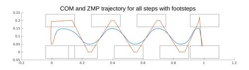
Fig. 10: Imposed ZMP trajectory (orange) and corresponding CoM (blue). The dashed rectangles represent the foot placements.
