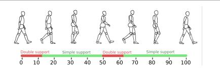
Fig. 1: SS and DS phase durations, measured as percentage of complete cycle.
