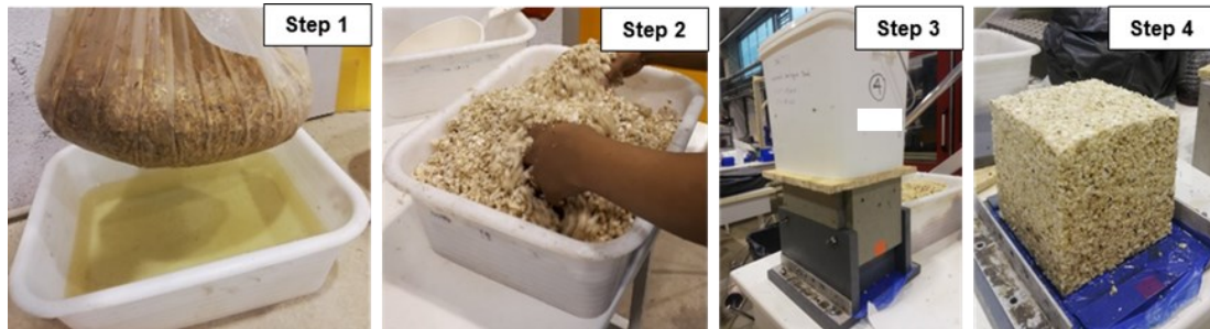
Fig. 2: Experimental protocol to measure wet compacted dry density and real water absorption
