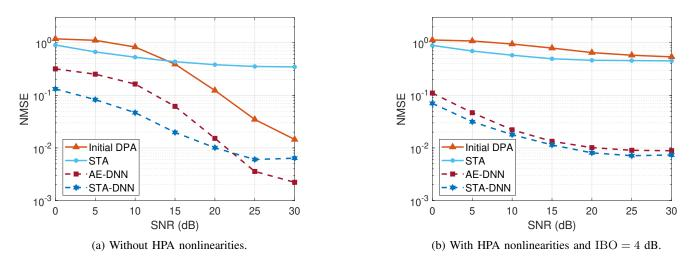
Fig. 3: NMSE performance in the IEEE 802.11p wireless communication scenario with v = 48 km/h.
