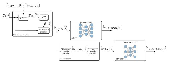
Fig. 2: Block diagram of the DNN-based estimators: AE-DNN and STA-DNN.
