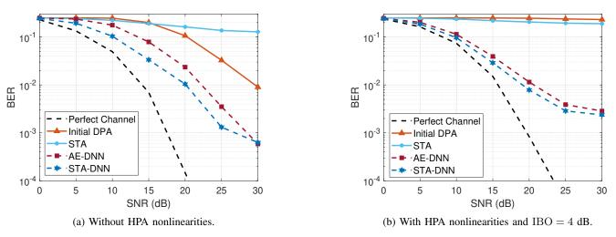
Fig. 4: BER performance in the IEEE 802.11p wireless communication scenario with v = 48 km/h.
