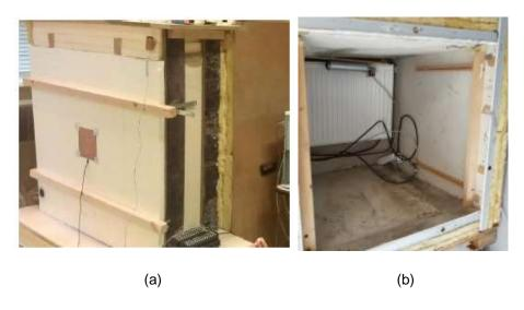
Figure 5- Photography of the tested wall (a) and the heating box (b)
