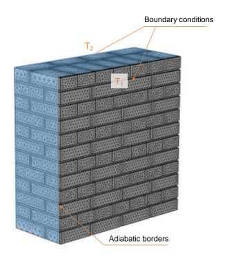
Figure 10- Boundary conditions for the numerical calculation of the equivalent thermal properties of masonry walls
