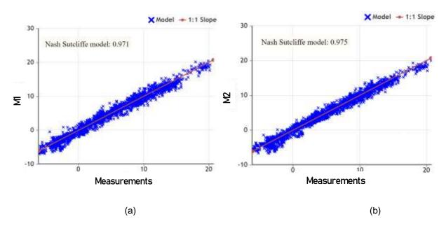
Figure 14- Nash Sutcliffe Efficiency coefficient (NSE) for Method 1 (a) and Method 2 (b)
