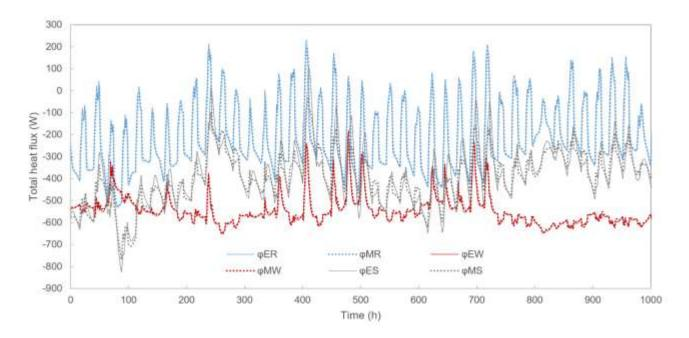
Figure 18- Total heat flux through the walls, the slab, and the roof for the MB and the EB
