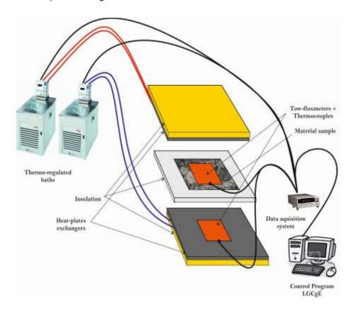
Figure 4- Thermal characterization setup for building materials
