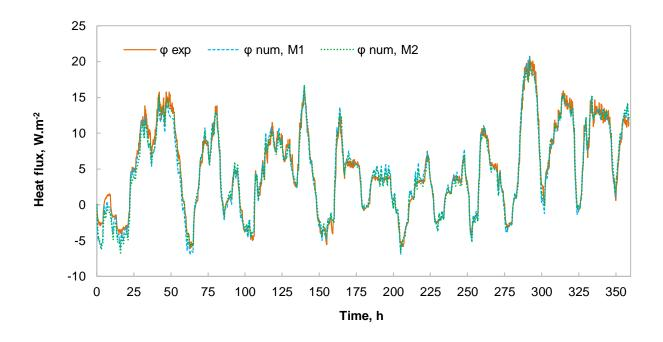
Figure 13- Comparison between experimental and numerical heat fluxes for the optimal solutions of the two methods
