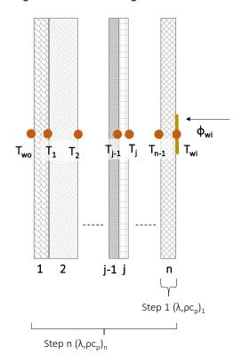
Figure 1- Sequential identification of multilayered walls
