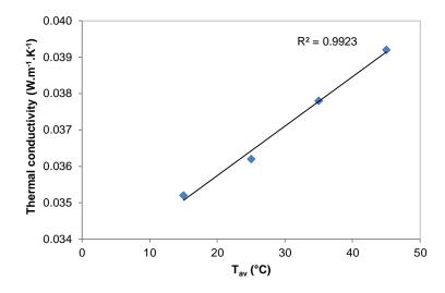
Figure 8- Thermal conductivity of the polystyrene sample for different temperature ranges
