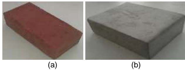
Figure 9- Characterized brick (a) and mortar (b) samples
