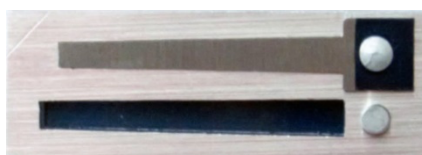
Figure 2: Bisonorous metal free reed with a double gap post-assembly: view from above. Photograph: Raffaele Pinelli, Osimo (AN), Italy, 2016.
