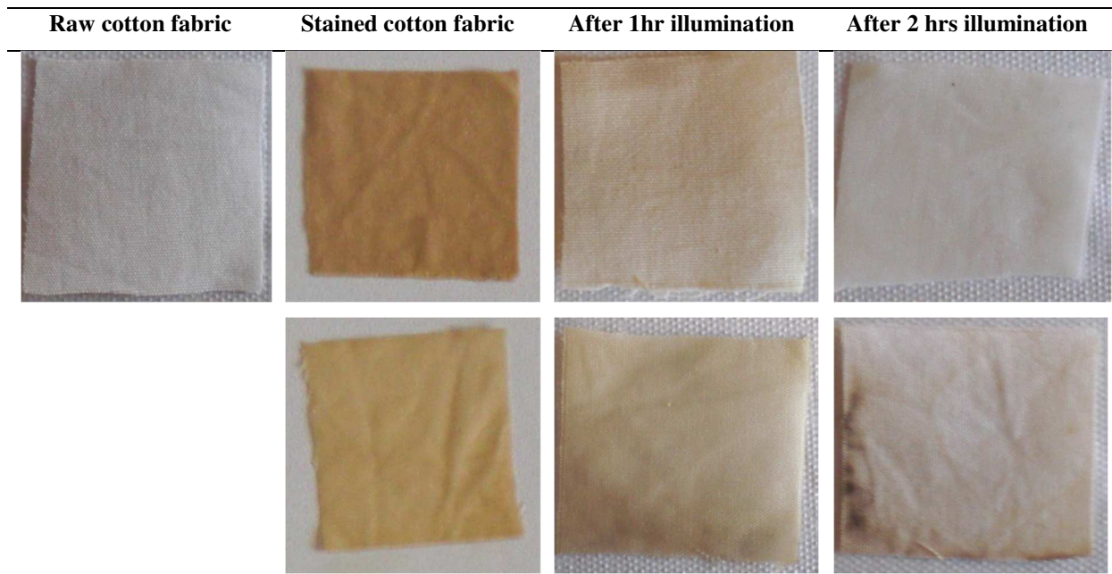
291 Figure 10. Self-cleaning performance of 1% Cu(II) doped TiO 2 calcined at 25 °C.
