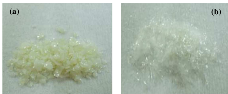
223 Figure 4. The images for (a) 5% Cu-doped TiO 2 and (b) non-doped TiO 2 NPs.
