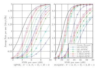
Fig. 6. Throughput in Rayleigh fading EQU4, U = 2 (for QPSK, 1 TI: dashed, 3 TIs: plain; for 16-QAM 0 TIs: dashed, 1 TI: plain).
