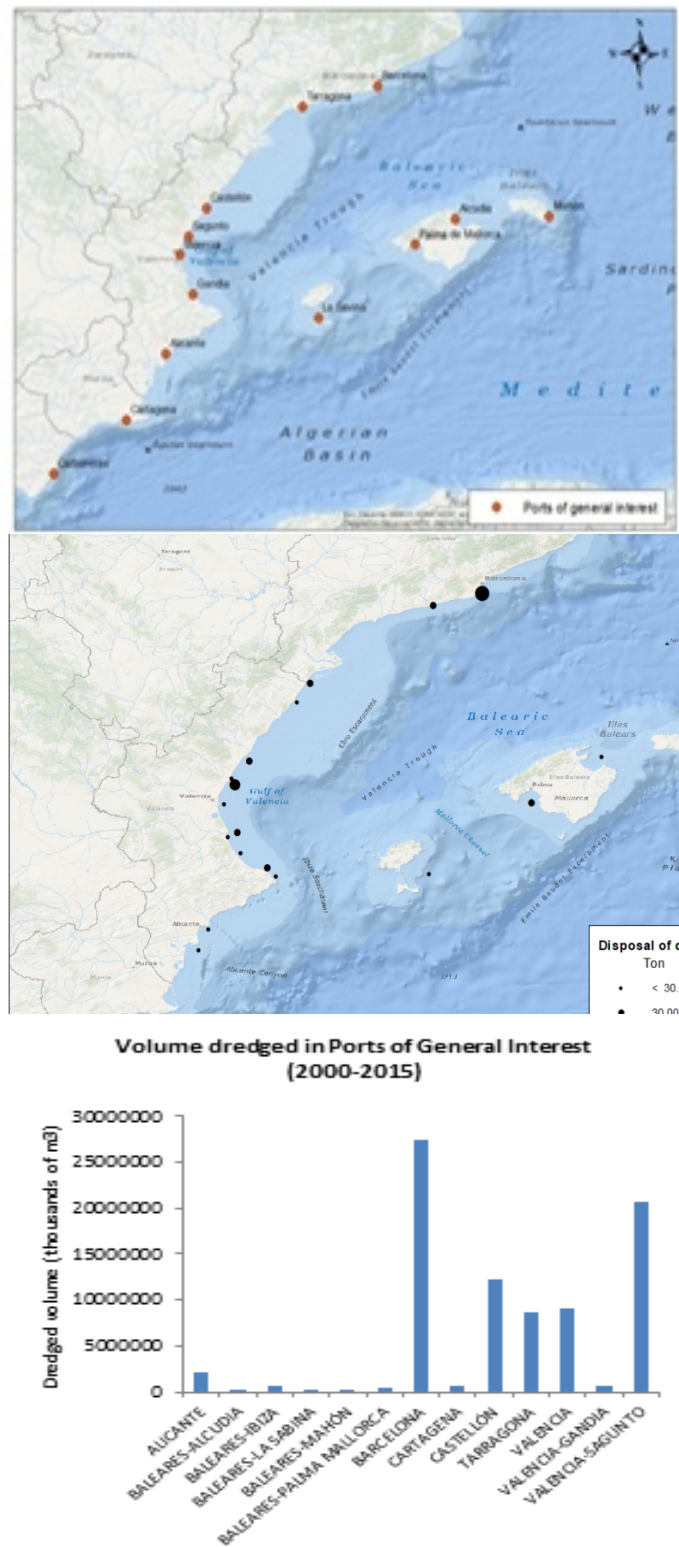
Figure 53,54,55 Geographical localization of ports of general interest, of disposal areas for dredged materials and volume dredged in Spanish waters.
