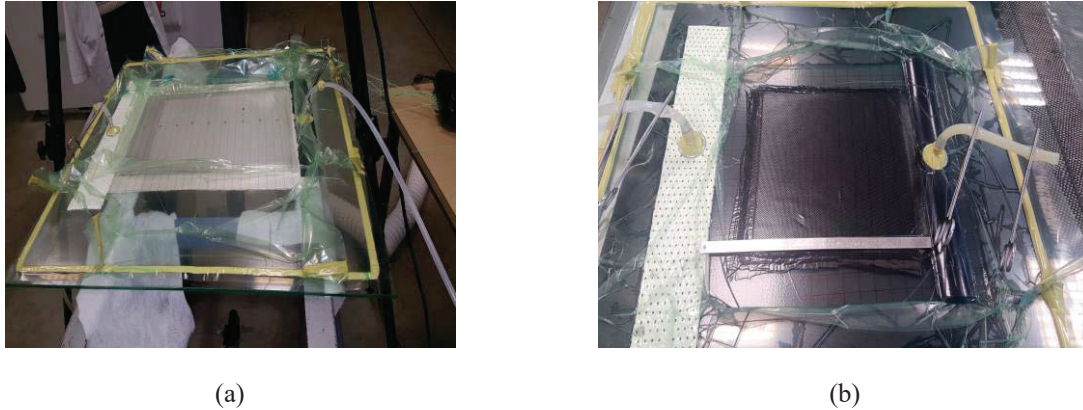
FIGURE 1. Manufacturing of composite specimen before (a) and after (b) the resin infusion
