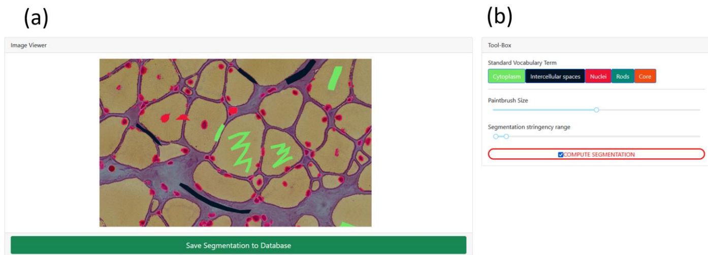
261 262 Figure 6: Screenshot of the image annotation module. (a) Image viewer used to navigate, 263 zoom and annotate the histology image. (b) Menu interface to select the annotation label, brush 264 width and segmentation parameters.
